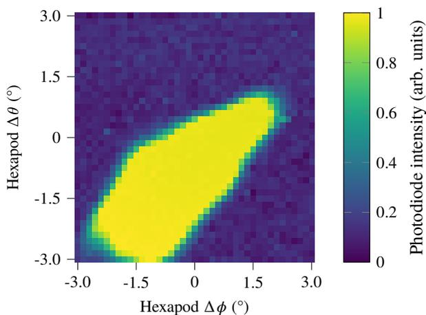
Figure 6: Normalized intensities for different fiber collimator rotations offsets at KARA beamline.
