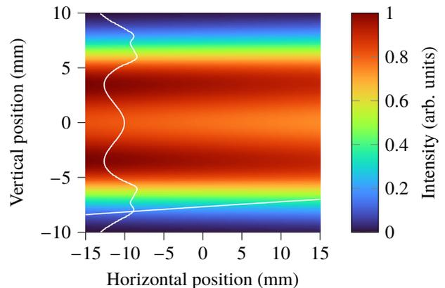
Figure 2: Transversal intensity profile of the bending magnet radiation before the synchrotron light port window (projections on the coordinate axis shown in white) at  $E = 500$  MeV and for  $\lambda = 700$  nm to 1600 nm.
