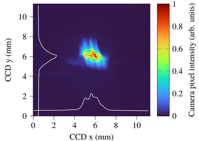
Figure 4: Intensity profile of the synchrotron radiation at the KARA beamline, taken at the collimator location.
