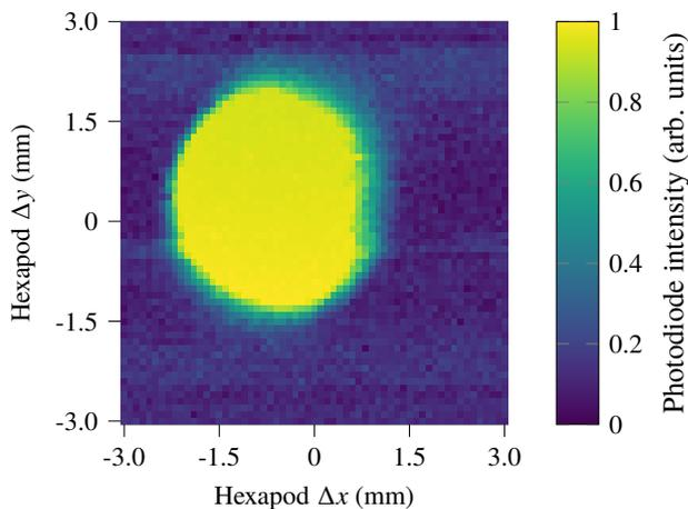
Figure 5: Normalized intensities for different fiber collimator position offsets at KARA beamline.
