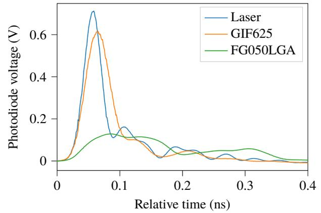
Figure 3: Optical pulses at laser output and after optical fibers; measured with DXM30BF photodiode (note: Laser only and GIF625 signals are limited by the  $\approx 30 \text{ ps}$  impulse responses of the 16 GHz digitizer used).
