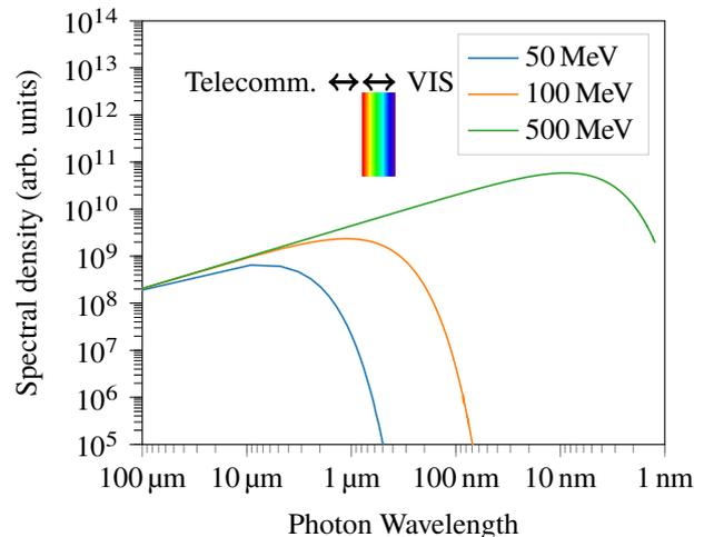
Figure 1: Spectral density of bending radiation at the booster dipole for different electron energies.
