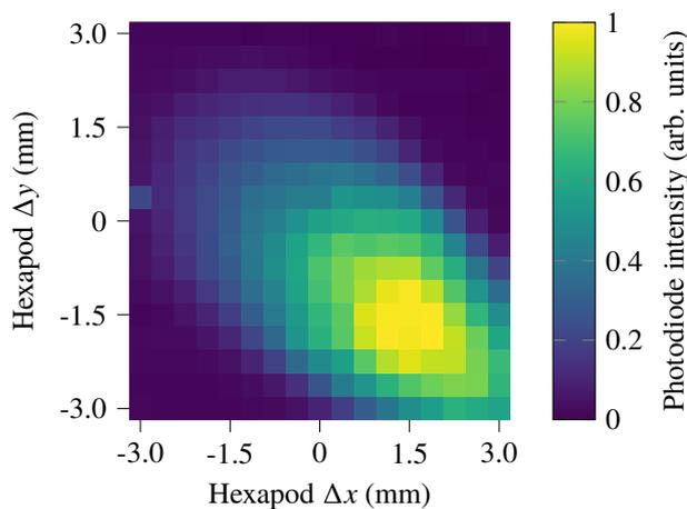
Figure 7: Normalized power meter values for different fiber collimator position offsets at KARA booster.
