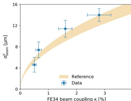
Figure 2: Measured vertical beam size at the NCD-SWEET beamline as a function of the ALBA coupling parameter. Adapted from [4].
