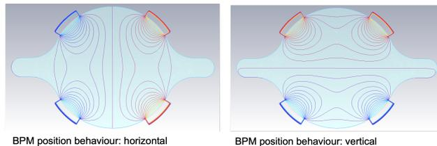
Figure 1: Lines of constant beam displacement of a FCC-ee main ring button BPM, horizontal (left), vertical (right).
