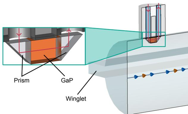
Figure 3: Conceptual design with two prisms attached to the crystal for an EOSD setup for FCC-ee [10].
