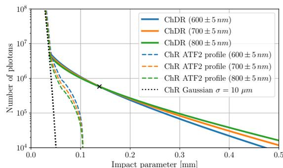
Figure 4: Expected photon yield according to the *non-stationary model*. Solid coloured lines correspond to ChDR at different wavelengths, dashed coloured lines correspond to the photon yield from direct Cherenkov radiation [20].
