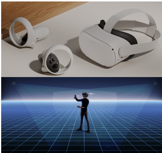
Figure 2.12: Stand-alone and stationary HMD concepts (meta 2022; HTC 2022)
