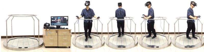
Figure 2.17: Hex-Core-MK1 omnidirectional treadmill (Z. Wang et al. 2022)
