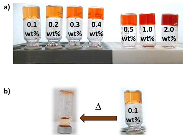
**Figure 2.** Supramolecular hydrogels made of **1** in phosphate-buffered saline (PBS) pH 7.4. a) Overview of the mechanical stability for samples in the concentration range 0.1–2 wt%. b) Heat-induced (>74 °C) gel shrinking (0.1 wt% **1** in PBS) with concomitant liquid ejection.
