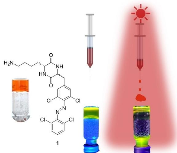
**Figure 1.** The hydrogel (orange) formed from **1** (here 0.3 wt%) in aqueous buffer can physically encapsulate cargo substances (yellow) and act as a molecular syringe. Upon irradiation with biocompatible red light (660 nm), the buffer with cargo is ejected from the gel, while in darkness the composition remains stable.
