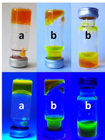
**Figure 5.** The fluorescent dye 5(6)-carboxyfluorescein (**2**) was added during the formation of a hydrogel (0.2 wt% of **1** in PBS at pH 7.4), and pictures were taken under ambient light or under UV irradiation. Sample **a** was equilibrated in darkness, sample **b** was irradiated for 4 h with red light (660 nm). In the latter case, the fluorescent cargo was predominantly released from the gel to the surrounding liquid and could be quantified.
