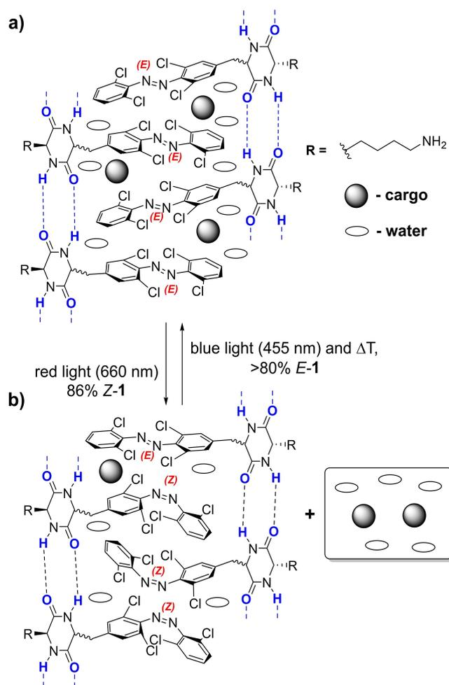
**Figure 6.** Schematic representation of the supramolecular fiber in the hydrogel loaded with cargo compounds (Figure 5). Hydrogel **a**) thermally equilibrated in the dark or **b**) irradiated with red light (660 nm).
