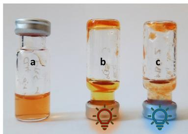
**Figure 3.** Hydrogel “a” formed from an equivalent mixture of diastereomers **1a** and **1b** (total conc. 0.1 wt%) was irradiated with red light (660 nm, 90 min) (sample “b”) causing gel shrinking with liquid ejection that was, however, not reversible upon irradiation with blue light (455 nm; sample “c”), even though the majority of the *E* isomer of **1** was restored under these conditions.
