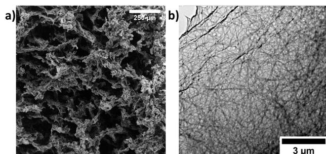
**Figure 4.** Electron microscopy imaging of the hydrogel samples prepared from **1** in PBS buffer at pH 7.4. a) SEM image of a xerogel composed of 1.0 wt% of **1**; scale bar: 250 μm. b) TEM image of a hydrogel composed of 0.1 wt% of **1**; scale bar: 3 μm.
