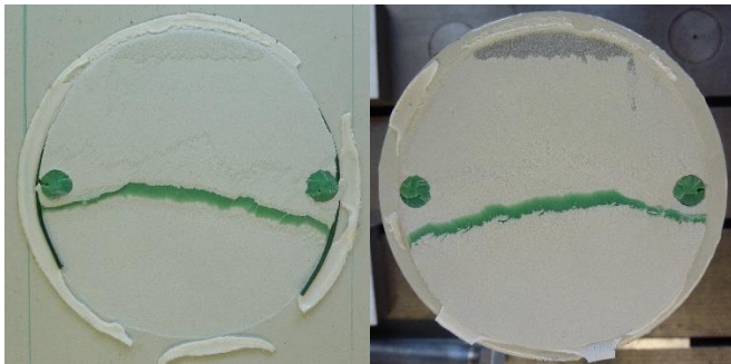
Figure 7 Exemplary fracture patterns for fasteners with end plate diameter of 100 mm
