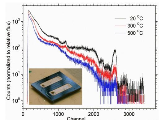
SiC detector without neutron converter at temperatures up to 500 °C.
