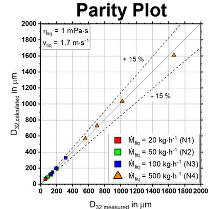
➤ Empirical model fits liquid mass flow between 20 and 500 kg·h<sup>-1</sup> with less than 15% deviation
