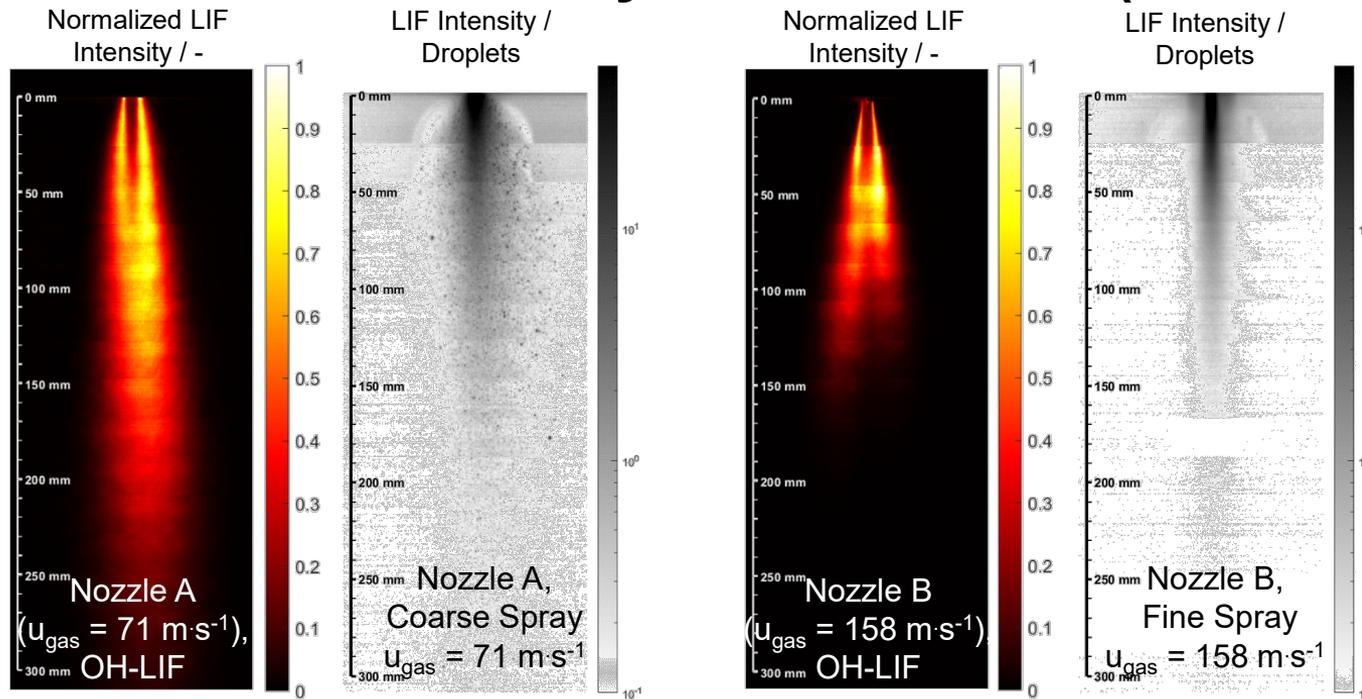
→ Different OH-distribution observed for different drop sizes and spray angles
