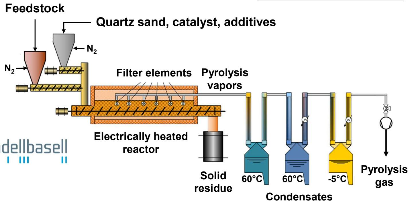
$$\dot{m}_{Feed} \approx 1 \text{ kg/h} \quad \frac{Sand}{Feed} \approx \frac{4 \text{ kg}}{1 \text{ kg}} \quad \frac{Catalyst}{Feed} \approx \frac{80 \text{ g}}{1 \text{ kg}} \quad \tau_{Solids} = 30-60 \text{ min} \quad T_{Reactor} < 600 \text{ }^{\circ}\text{C}$$
