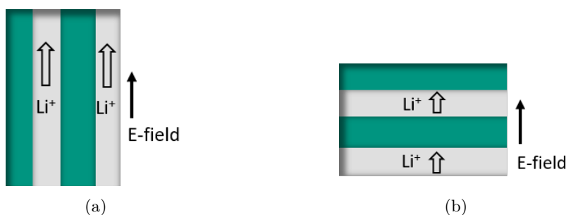
Figure 6.1: Schematic representation of ion conduction in an (a) perpendicular and (b) parallel orientation on the example of \text{Li}^+ . The ionic conductivity should increase with a perpendicular orientation and decrease with a parallel orientation because the direct path to the electrode is blocked by the non-conducting layers.
