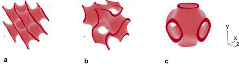
Fig. 1. Examples of TPMS unit cells: a. Diamond; b. Gyroid; c. Primitive.
