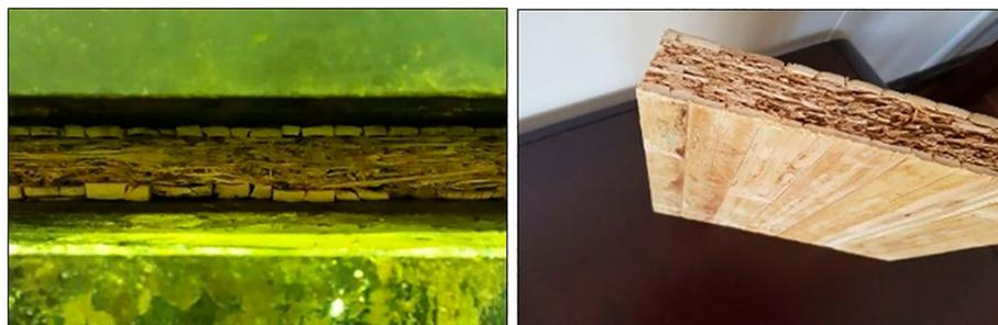
**Figure 4.** Three layers (core- two outer layers) of sandwich panel under the pressure.
