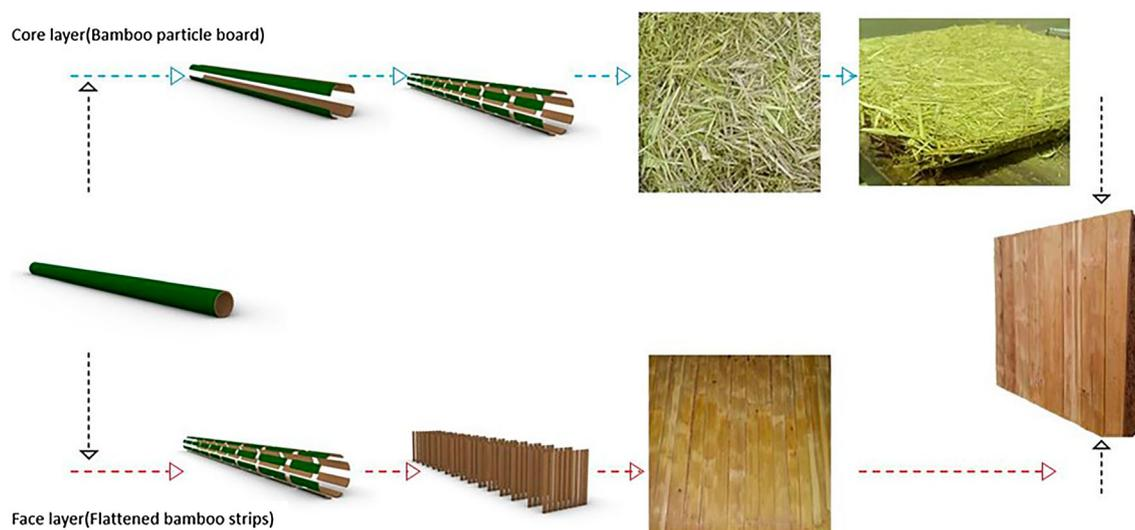
**Figure 3.** The panel production process in schematic form.
