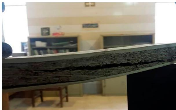
**Figure 8.** Failure of the core layer due to the compression load.
