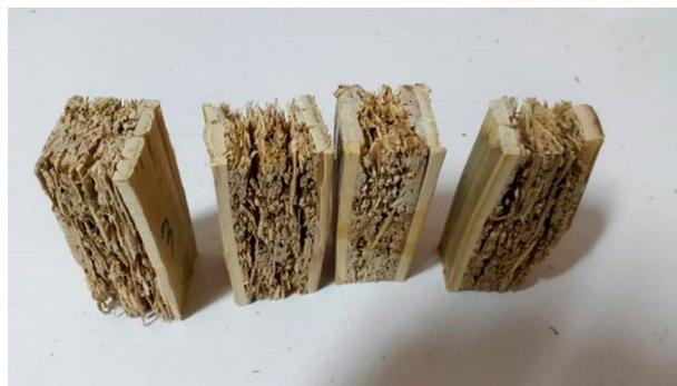
Figure 10. Sample failure modes in compression test parallel to the face grain.
