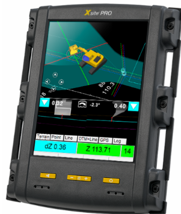
Figure 7. Xsite ® PRO 3D system that is installed in the excavator cabin [42].
