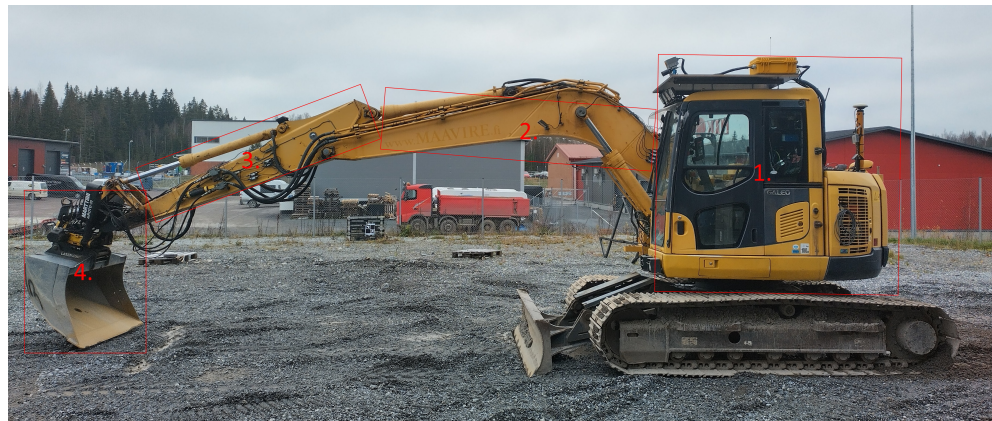
Figure 12. Excavator used in data collection. In the picture, the cabin (1.), boom (2.), arm (3.), and bucket (4.) are highlighted with red boxes [4].
