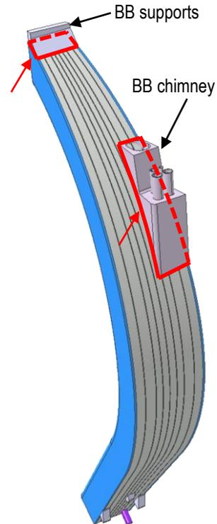
11. Chimney and segment supporting structures assembly TIG weld
