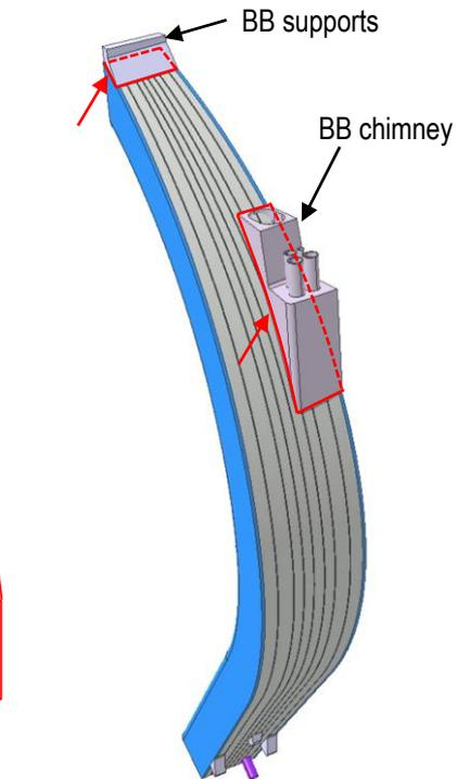
6. TIG weld of chimney (welds act against in-VV LOCA) & BB supports to BB backplate.
