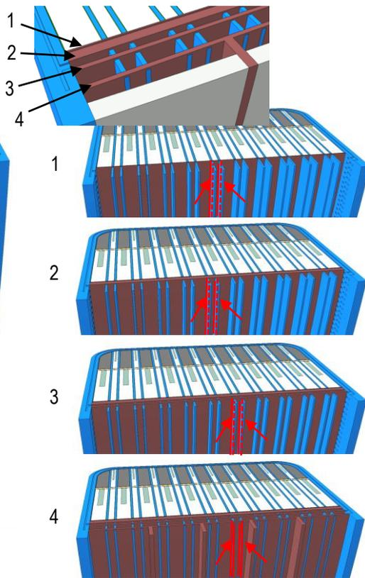
3. Insertion of front thick cassettes, weld of thick stiffener stripes and insertion of back thick cassettes
