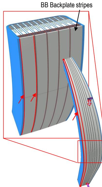
5. TIG/laser weld of BB backplates to manifold stiffeners, FW & caps. Welds act against in-VV LOCA
