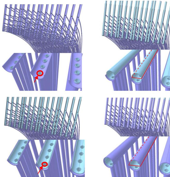
1. Manufacturing of double bundle tubes (planar curvature)
