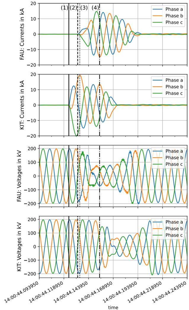
FIGURE 20. Short-circuit simulation directly at the coupling point
