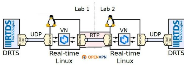
FIGURE 17. Set up of the distributed co-simulation
