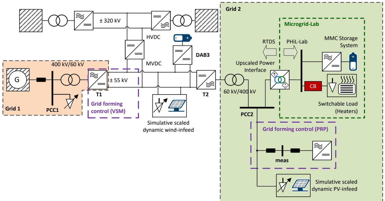
**FIGURE 6.** Basic structure of the MVDC/HVDC test system
