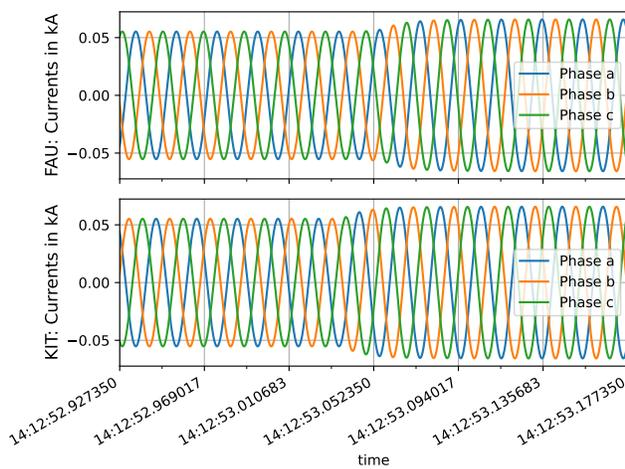
FIGURE 18. Load change at KIT side
