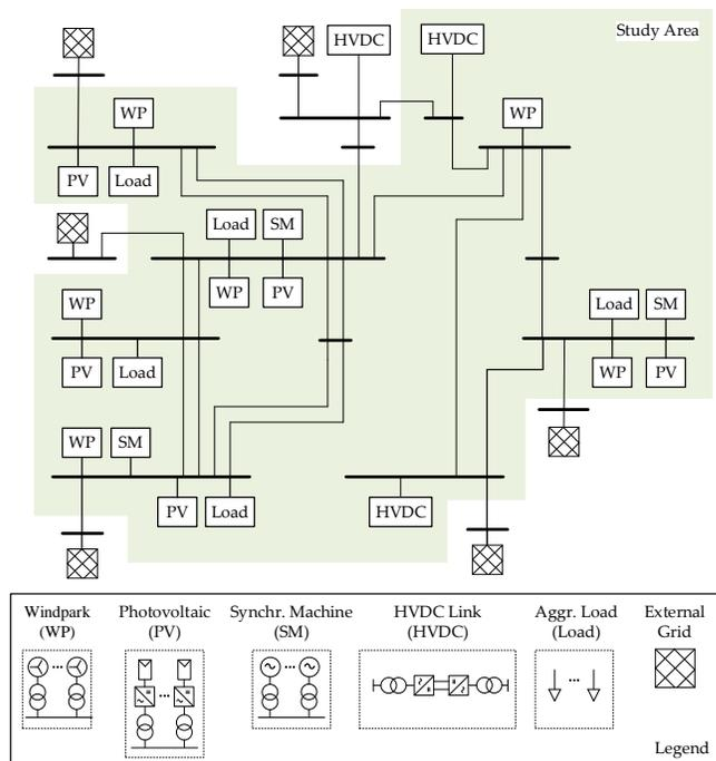
FIGURE 3. Schematic single line diagram of real-time model
