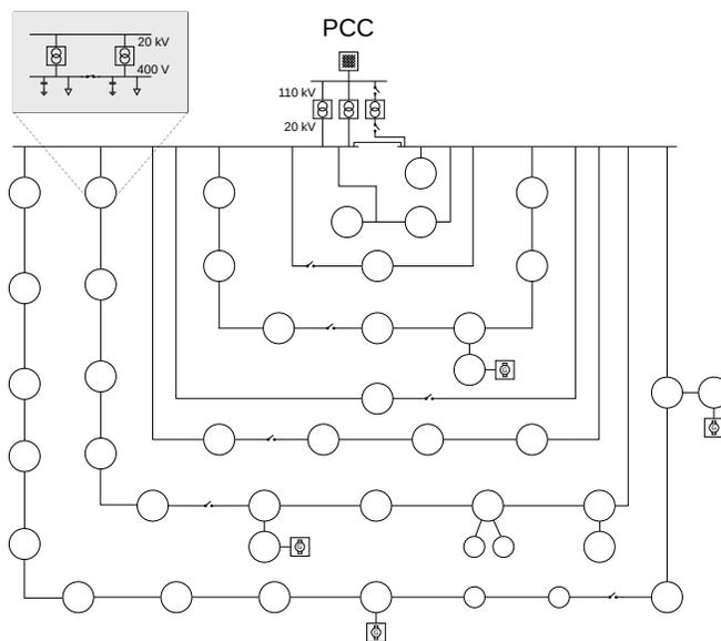
FIGURE 4. Single line diagram of the RSCAD model of the Campus North 20 kV grid.
