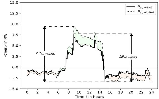
FIGURE 5. Resulting power with and without energy hub integrated into the grid model for an exemplary day [27]
