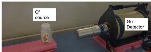
Figure 2. Experimental setup for the measurement with the old source and a HPGe detector.
