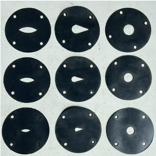
(a) Photograph of the polyvinyl chloride film cutted MROPs in the sizes S, M and L.
