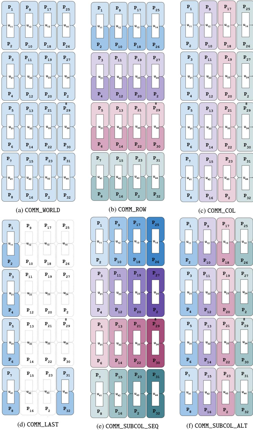
Figure 4.4.: Communicator groups when the number of collocation points is  $M = 4$  and the number of time steps is  $L = 4$ . The parallelization strategy used is  $n_{\text{step}} = 4$ ,  $n_{\text{coll}} = 4$  and  $n_{\text{space}} = 2$ .
