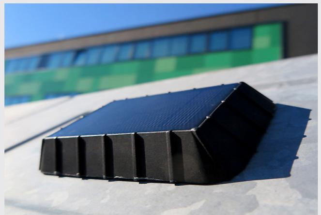
Sensors in or on waste containers measure parameters such as temperature, motion, sound or geographical position. From this, information on the fill level, the respective position or anomalies (e.g. fire, theft) can be derived.
