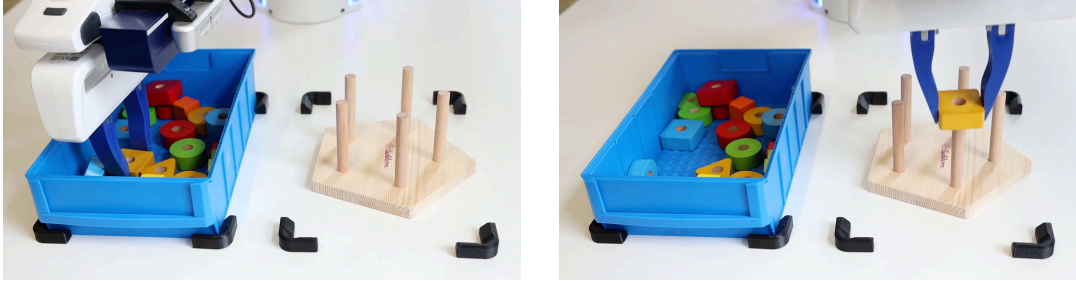
Figure 6.1: A pick-and-place action with a grasp (left) and the subsequent place (right).
