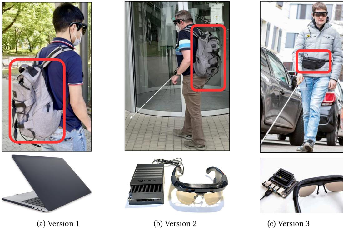
Figure 58: Three different versions and iterative development of the *Vision4Blind* system. The versions from left to right are: (a) using a heavy laptop in a backpack, (b) using an NVIDIA Xavier Jetson AGX Xavier processor in a backpack, and (c) using a lightweight NVIDIA Jetson Nano processor in a portable belt bag with an on-device user interface.
