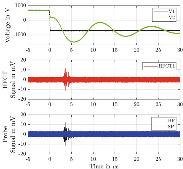
**Fig. 8** PD measurement at stator with falling edge in envelope mode
