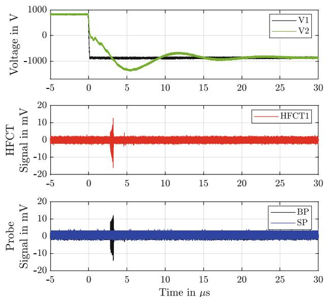
**Fig. 9** PD measurement at motor with falling edge in envelope mode
