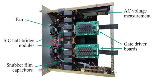
Fig. 1 Photo of the SiC inverter in a 19" rack-mount chassis
