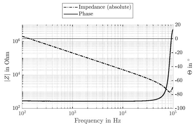
Fig. 6 Frequency response of absolute impedance and phase measured at the stator
