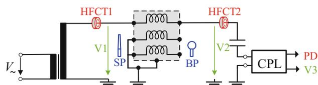
Fig. 2 Experimental setup for 50 Hz sine wave voltage
