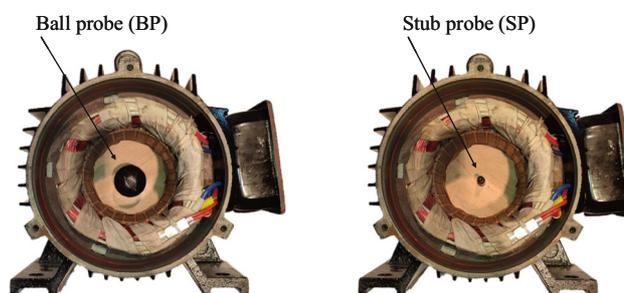
Fig. 4 Positions of the near-field probes in the stator. **a** ball probe, **b** stub probe
