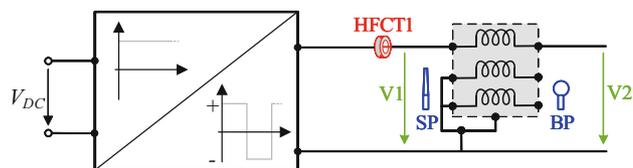
Fig. 3 Experimental setup for 1 kHz square wave voltage
