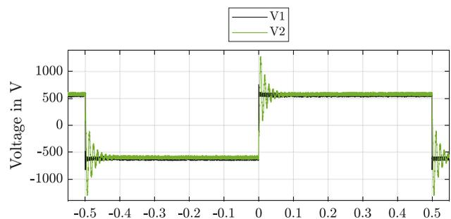
Fig. 7 Measured voltage waveform at the stator
