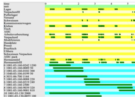
**Figure 5.** Utilization of the stations and processing span of the orders.
