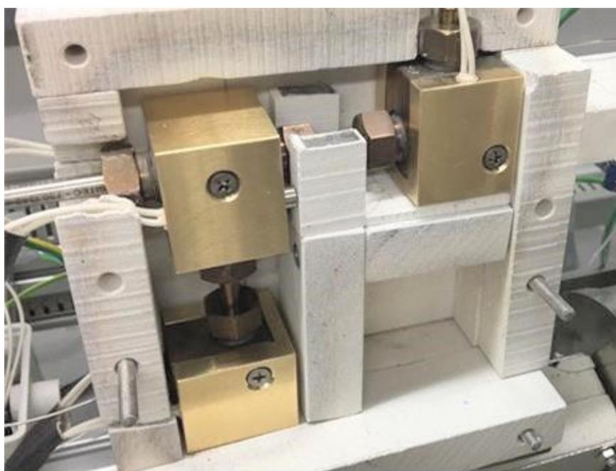
Figure 4-2: Mixing unit with opened insulation housing.
