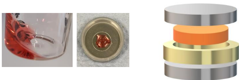
FIGURE 35: LEFT: Representative pictures of a fluid electrolyte in a glass vial MIDDLE: Picture of the lower cell case with one stainless-steel electrode, the ring spacer and a drop of electrolyte. RIGHT: Schematic representation of the cell assembly showing the stainless-steel electrodes in metallic color, the ring spacer in yellow color and the fluid sample in orange color.
