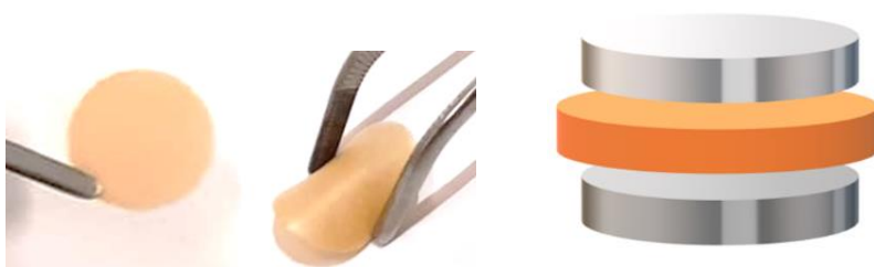
FIGURE 34: LEFT AND MIDDLE: Representative pictures of an electrolyte membrane RIGHT: Schematic representation of the cell assembly showing the stainless-steel electrodes in metallic color and the membrane in orange color.
