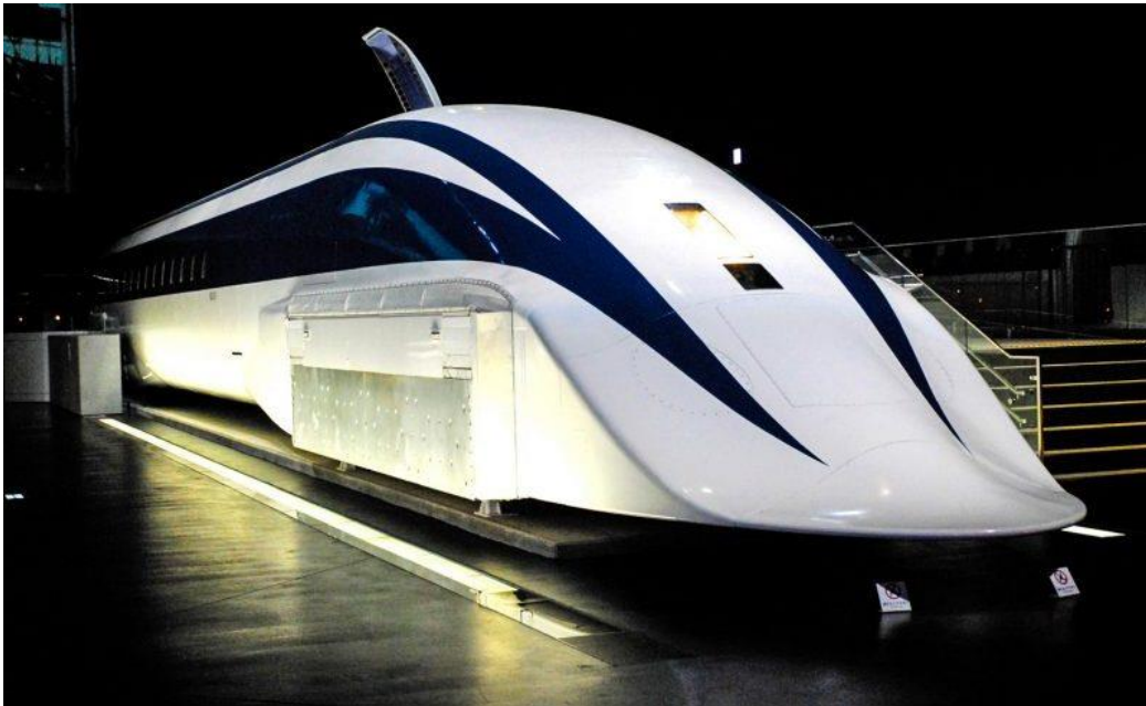
Yamanashi: Japanese low- T_c superconducting maglev train
