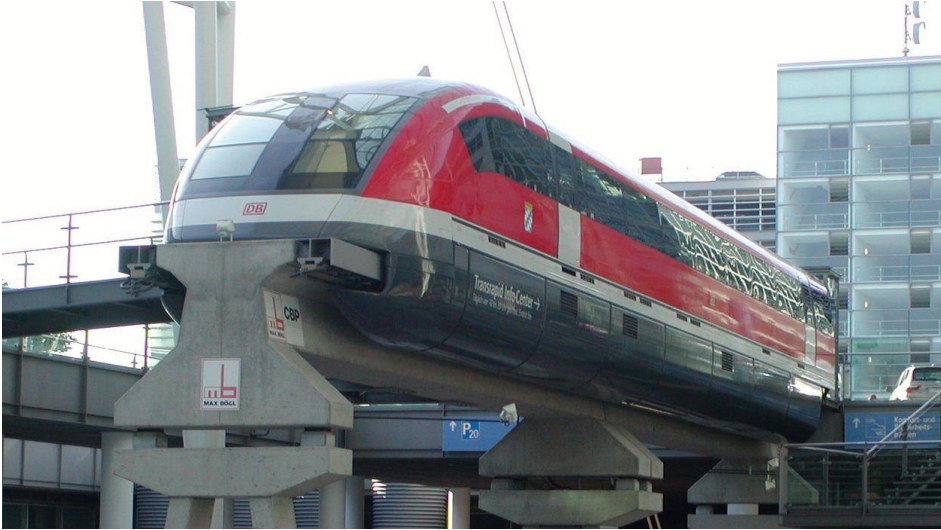
German Transrapid TR-07 Electromagnetic Levitation (EML)
