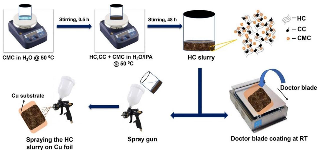
Scheme 1. Preparation scheme of spray-coated HC electrodes.
