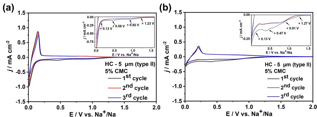
Figure 2. CVs of spray-coated HC electrodes with 5% binder (5 μm (type II)). (a) In 1 M NaClO<sub>4</sub> in PC, (b) 1 M NaClO<sub>4</sub> in PC/2% FEC. Scan rate: 0.1 mV s<sup>-1</sup>, potential range 0.01–2.00 V vs. Na<sup>+</sup>/Na.
