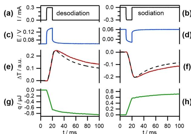
**Figure 5.** Current (black), potential (blue), temperature (red), and heat (green) transients upon pulsed discharging (a, c, e, g) and charging (b, d, f, h) of a 20 μm thick HC film by 10 ms positive and negative current pulses with 300 μA amplitude, respectively. In addition, the thermal response of the electrode to a 10 ms laser pulse is shown as a black dashed line. The amplitude is adjusted to the extremum of the respective temperature transient.
