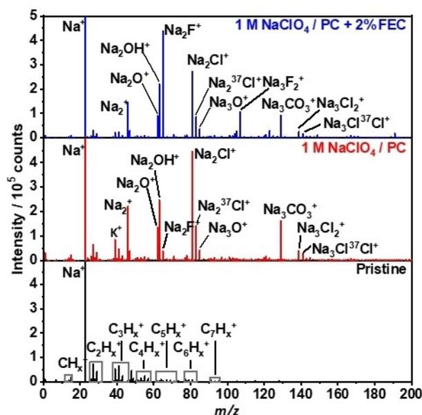
**Figure 4.** Exemplary ToF-SIMS surface spectra in positive secondary ion mode of the sample cycled in PC and 2% FEC (blue), the pristine sample (black) and the sample cycled in PC (red). The spectra are being displayed as line spectra with respect to the peak areas.
