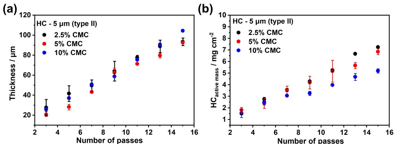
Figure 1. Thickness and mass loading of spray-coated HC - 5  $\mu\text{m}$  (type II) composite electrodes. (a) Thickness of spray-coated HC composite electrodes. (b) Active mass loading per  $\text{cm}^2$  with 2.5%, 5% and 10% binder. Number of passes: 3 to 15 passes. Error bars reflect three different samples with three measurement spots per sample ( $n=3$ ).
