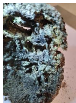
Figure 4: Sinter bed formed during sugarcane straw gasification with O 2 and water steam as gasification agent.
