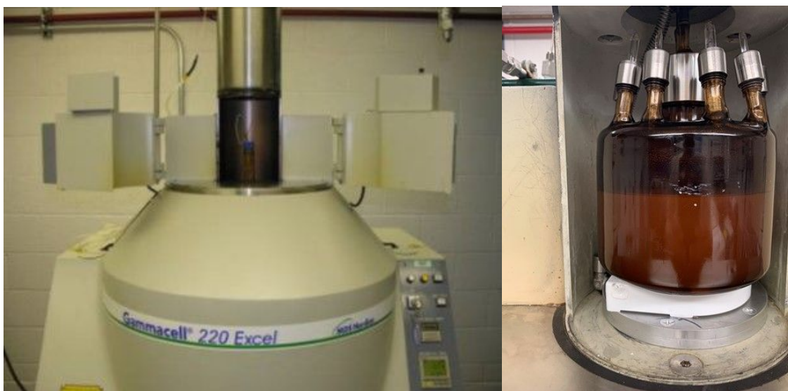
Figure S3. MDS Nordion GammaCell 220 Excel gamma irradiator (left). Re-designed test loop irradiation vessel installed in sample chamber (right).
