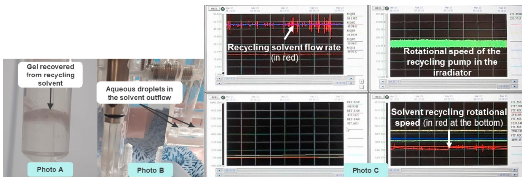
Figure 6. Photo A: gel recovered in the recycling solvent vial and in the flow meter. Photo B: droplets collected in the solvent outflow. Photo C: screenshots showing continued instability in the recycling solvent flow rate and pump speed during the Marcel loop test.
