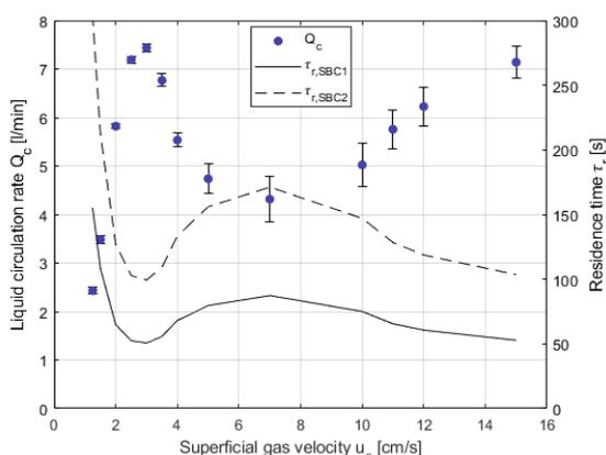
Fig. 2: Impact of superficial gas velocity  $u_s$  on liquid circulation rate  $Q_c$  with standard deviation and residence time  $\tau_r$  in SBC 1 and 2.
