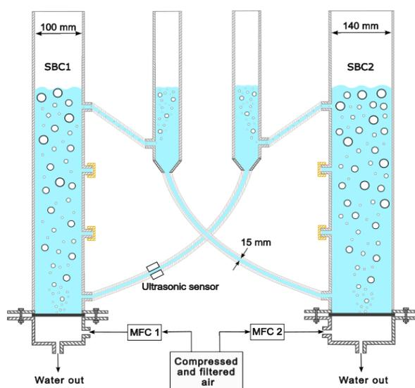
Fig. 1: Cold flow model of connected SBC as new reactor concept for the SE FT synthesis.
