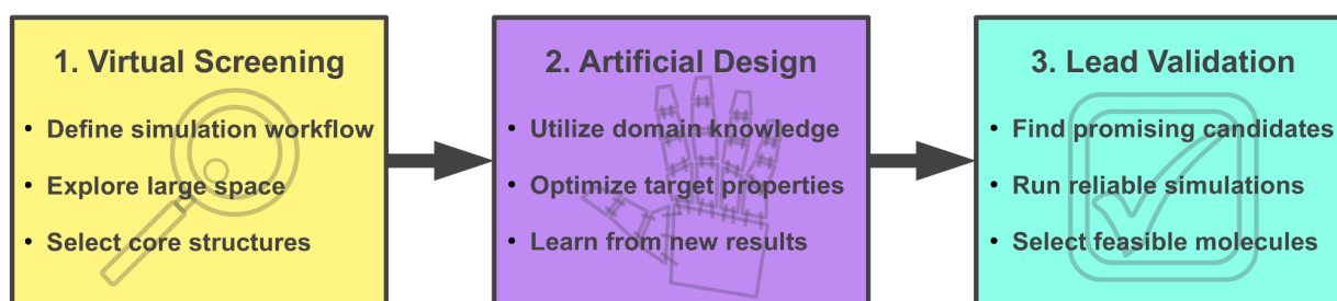
Figure 1. Accelerated molecular discovery workflow adopted in this work starting from high-throughput virtual screening, proceeding to artificial molecular design via a genetic algorithm enhanced by neural networks and filters based on domain knowledge, and finishing with lead validation.
