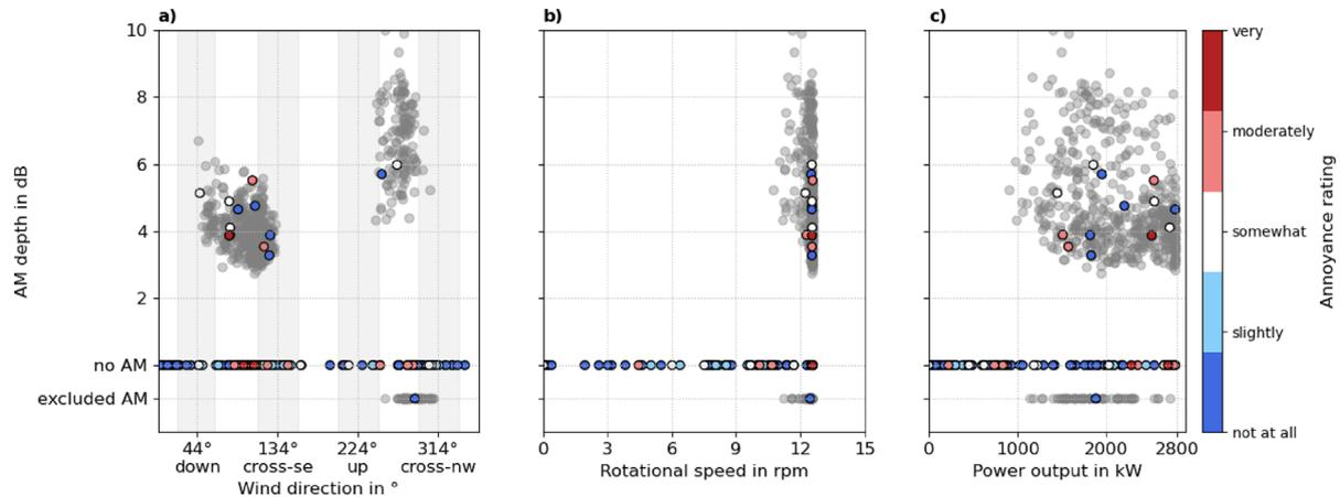
**Figure 22.** All AM depth data from the building location for (a) wind direction, (b) rotational speed and (c) power output of WT 2 in grey with color-coded annoyance levels from residential noise reports. Reports occurred during AM occurrence, no AM and AM excluded due to filtering.
