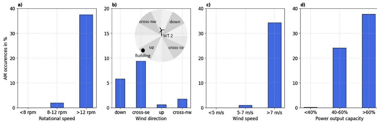
**Figure 19.** Normalized AM occurrence detected with IOA method from 2022/03/24 to 2022/05/11 at the building location for different WT operational parameters from WT 2 at hub height. (a) Rotational speed, (b) wind direction, (c) wind speed and (d) power output capacity.
