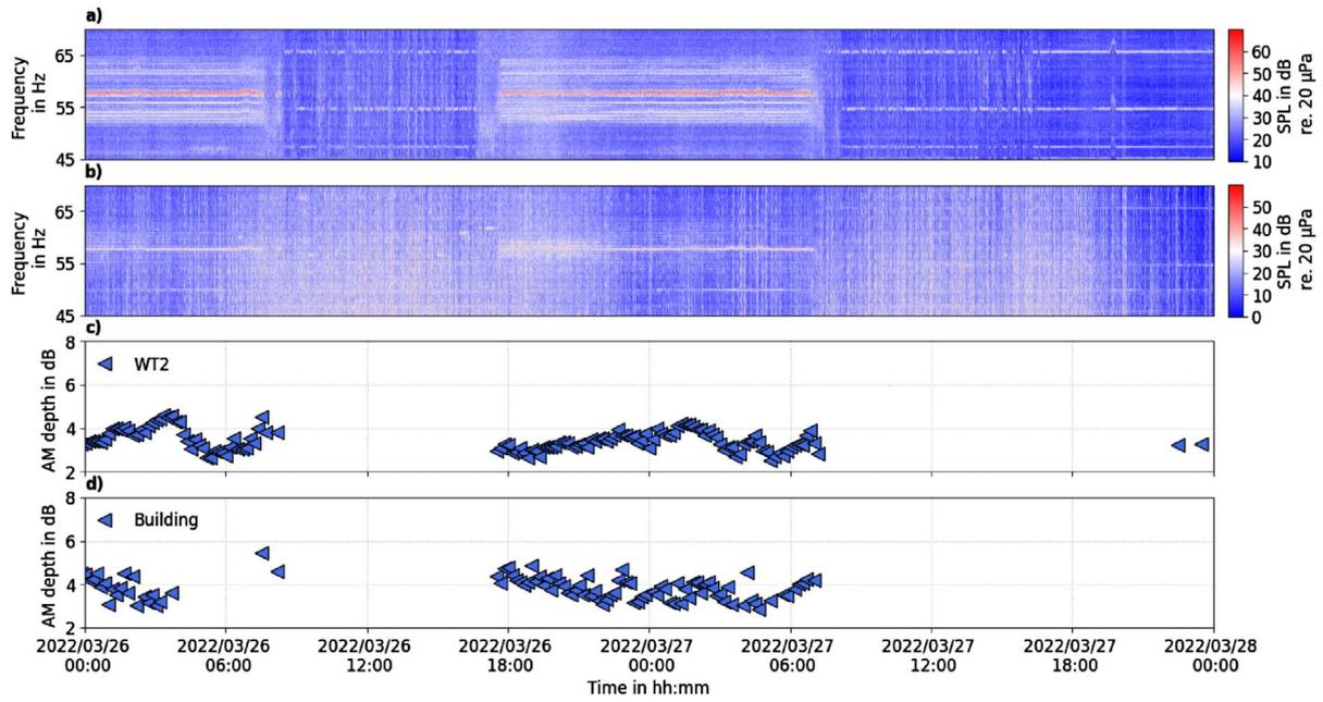
**Figure 9.** SPL spectrogram showing the presence of AM of multiple tones on 2022/03/26 and 2022/03/27. AM can be identified by horizontal lines around the carrier tone spaced at the BPF (modulation frequency). (a) Wind farm location, (b) outside the building at 1 km distance, (c) and (d) detected AM samples for rated rotational speed of WT 2 at the wind farm and building location.
