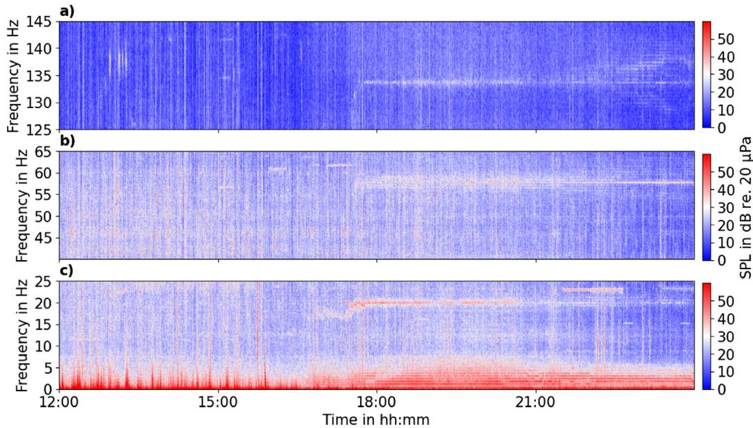
**Figure 7.** SPL spectrogram showing the presence of AM of multiple tones on 2022/03/26 in 1 km distance to the wind farm. AM can be identified by horizontal lines around the carrier tone (57.8 Hz and 133 Hz) spaced at the BPF (modulation frequency) in the evening hours between 18:00 and 24:00 UTC.
