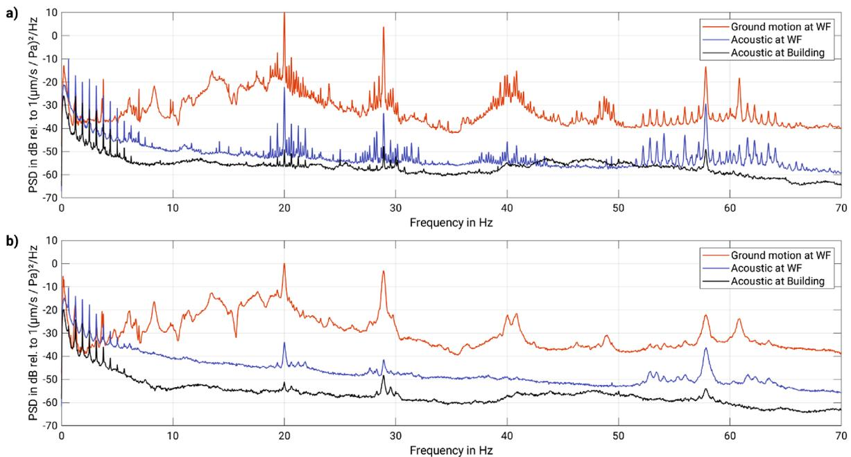
**Figure 10.** Spectra of acoustic and ground motion data for 2 time windows from 2022/04/21 with clear (top, 0:00–6:00 UTC) and no (bottom, 19:00–24:00 UTC) AM. While the peaks at 20 Hz and 29 Hz exhibit side peaks at distances of 1/3 of the BPF, the peak at 57.8 Hz shows side peaks at the BPF. A further main peak is observed at 61 Hz in the ground motion data, which is smaller relative to the amplitude of the surrounding frequencies in the acoustic data.
