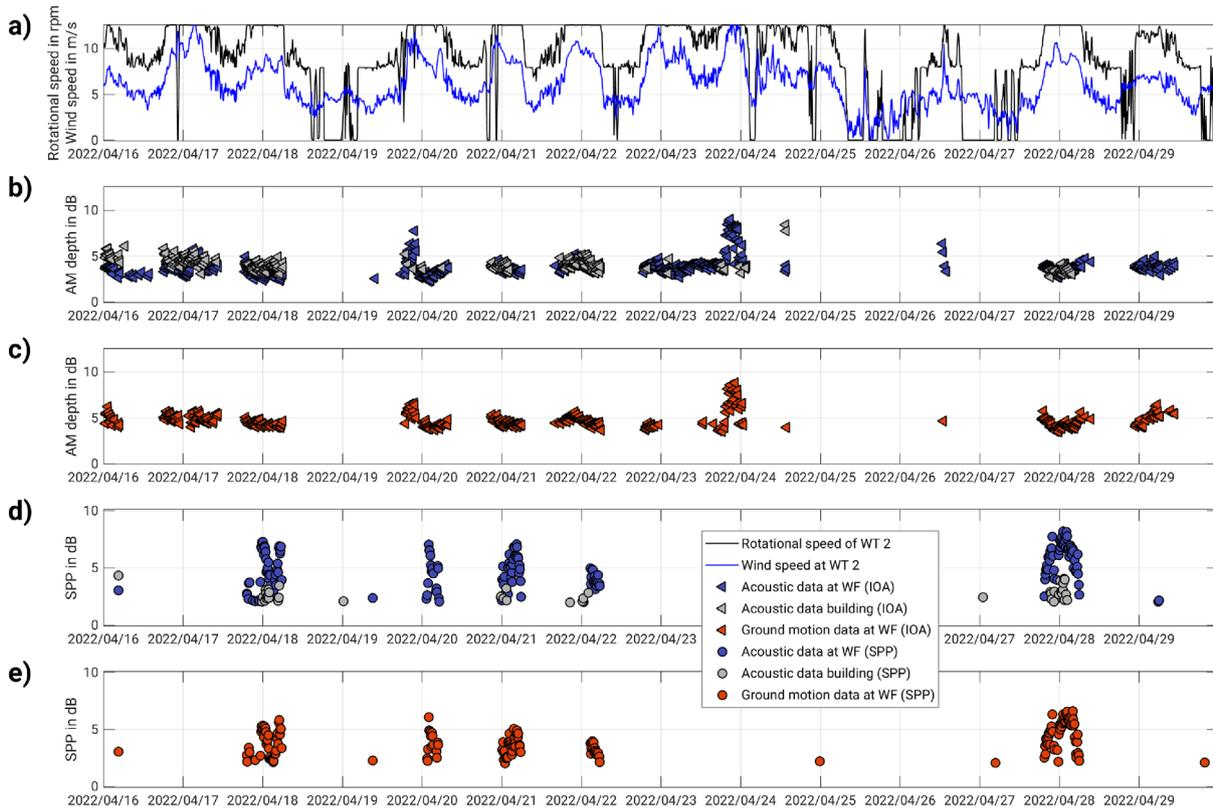
**Figure 14.** (a) Rotational speed and wind speed data for WT 2 of wind farm Tegelberg. (b)–(e) Results for valid AM detection from 2022/04/16 to 2022/04/29 for the (b)–(c) IOA as well as the (d)–(e) SPP methods for acoustic (blue/grey symbols) and ground motion data (red symbols).
