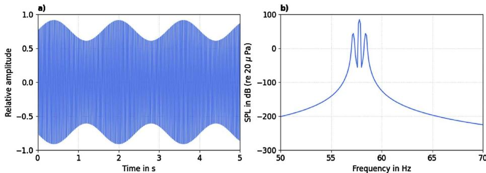
**Figure 1.** AM signal for carrier tone of frequency 57.8 Hz and modulating tone of frequency 0.625 Hz, (a) over time and (b) over frequency with side peaks spaced at 0.625 Hz.
