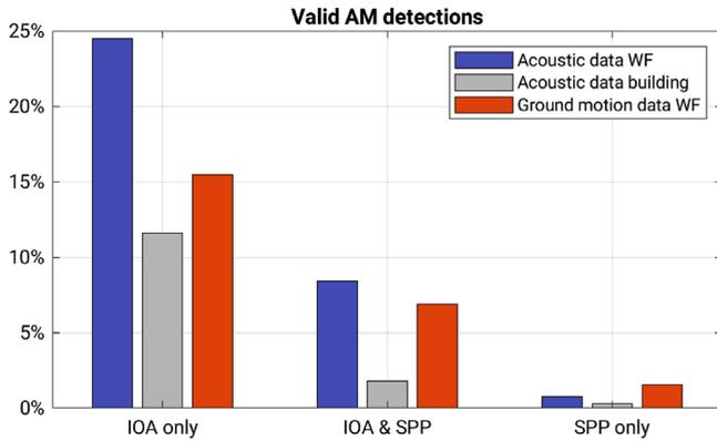
**Figure 15.** Comparison of AM detection results for all 10-minute time windows from 2022/04/16 to 2022/04/29. Percentage of AM detections with either the IOA or the SPP method only (left and right columns) or AM detected with both methods simultaneously (middle column). In this period, rated WT operation (rotational speed  $>12$  rpm) was reached in 32% of the total 10-minute time windows.
