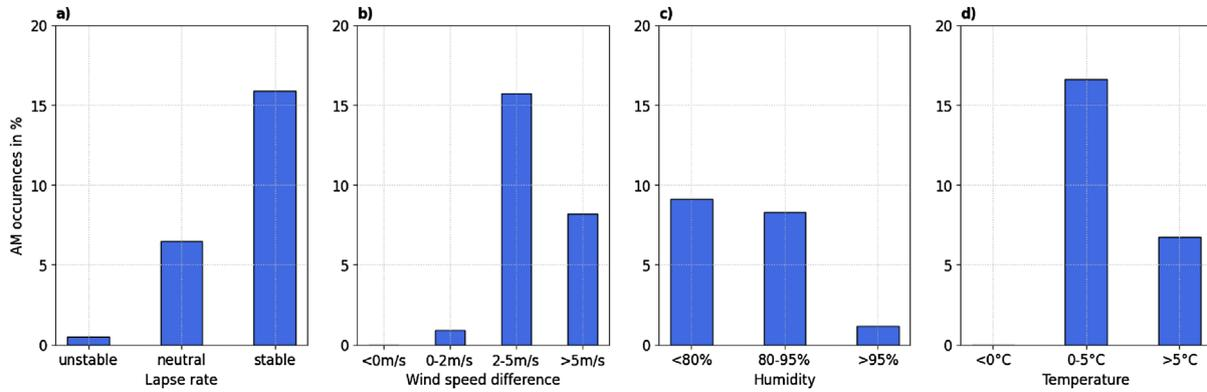
**Figure 18.** Normalized AM occurrence detected with the IOA method from 2022/03/24 to 2022/05/11 at the building location for different meteorological parameters from the WINSENT test site. (a) Lapse rate indicating unstable, neutral and stable atmospheric conditions, (b) wind speed difference for wind speeds at 11 m and 98 m, (c) humidity in 3 m height and (d) temperature in 3 m height.
