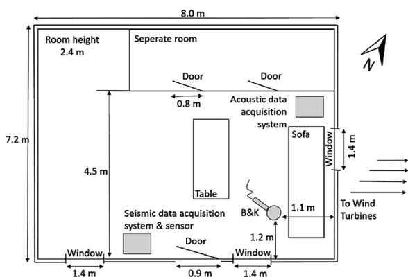
**Figure 4.** Sketch showing the instrumentation set-up inside the building. Exterior facades are marked with a double line.
