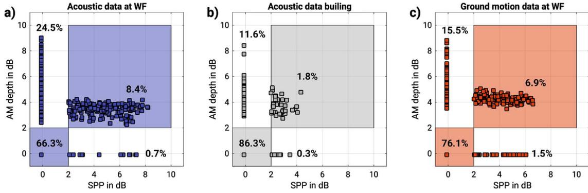
**Figure 16.** AM depth vs. SPP for all considered time windows from 2022/04/16 to 2022/04/29 for (a) acoustic data from the wind farm, (b) acoustic data from the building location, and (c) ground motion data from the wind farm. The displayed percentages add up to the numbers shown in Figure 15 and Table 5 and shaded areas highlight regions with detections or nondetections consistent between both methods.
