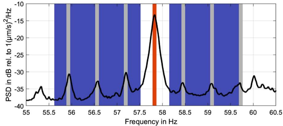
**Figure 11.** Ground motion spectrum centered at 57.8 Hz from 2022/04/21 0:00–6:00 UTC with clear AM. The difference of the arithmetic means of the grey and blue colored frequency areas in dB are taken to calculate the prominence of the side peaks.
