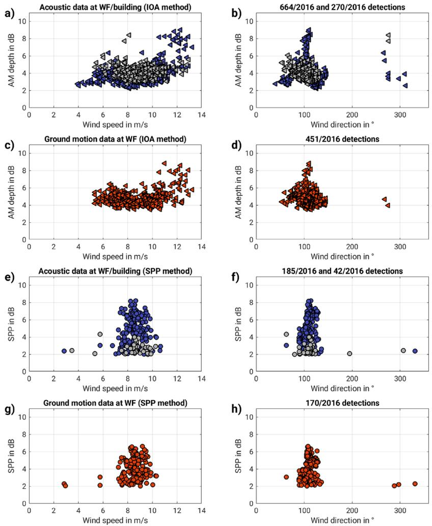
**Figure 17.** Results for AM detection in acoustic (blue and grey symbols) and ground motion (red symbols) data for 2022/04/16–2022/04/29 versus wind speed (left column) and direction (right column) using the (a)–(d) IOA and (e)–(h) SPP methods. Blue symbols show results for measurements at the WF and grey for those at the building location.
