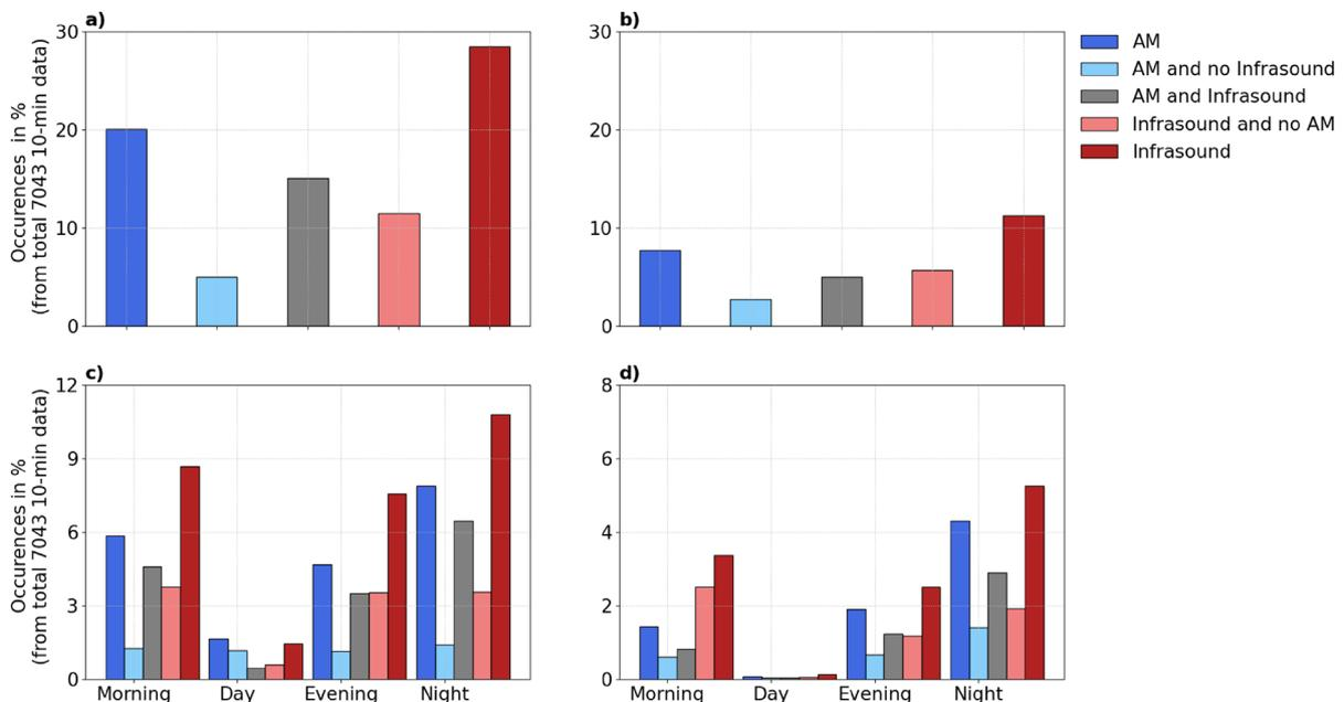
**Figure 20.** AM and infrasound occurrence from 2022/03/24 to 2022/05/11 for the (a) wind farm and (b) building location. Variation of AM and infrasound during day and night time for the (c) wind farm and (d) building location.
