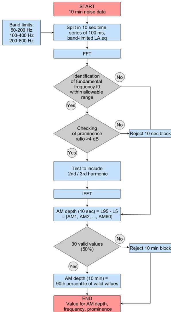
**Figure 8.** Flowchart for detection of AM with the IOA reference method.
