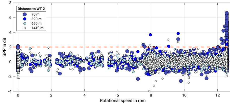
**Figure 13.** SPP over rotational speed for all considered 10-min time windows at the four ground motion measurement sites shown in Figure 2. The detection threshold for AM is set to 2 dB for the SPP method, indicated by the red dashed line. Lower SPP values occur for all rotational speeds and, therefore, only above this threshold detections are reasonable. Only at the site in 70 m distance to WT 2 SPP values of more than 2 dB are observed for multiple time windows.
