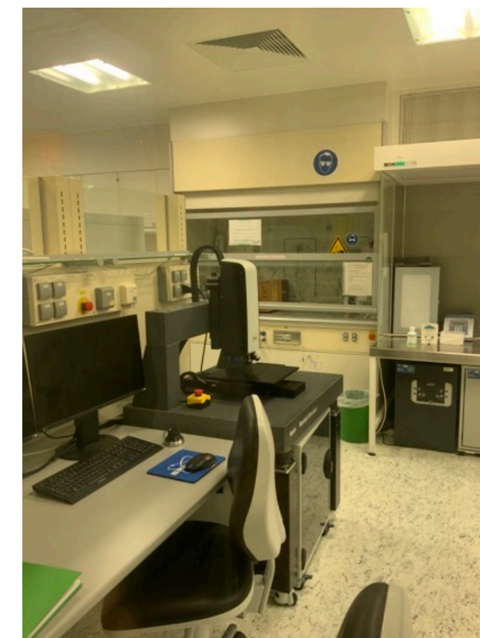
Vertical Light Interferometer, courtesy of R. Thelen
