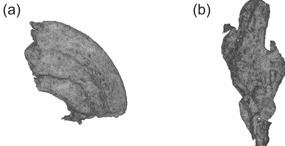
Fig. 9. 3D models of FLUFF particles. (a) plastics: 3D plastic particle (b) foils: 2D plastic foil.
