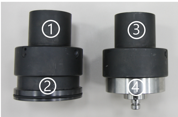
Figure 3.2: The two piezo electro-acoustic transducers by the company GL Testsystems (1 and 3) [3], with a round contact surface diameter of 80 mm attached to their adapters (2 bottom and 4 top).
