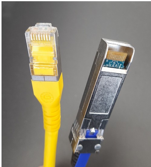
Figure 2.4: Two typical plug standards for network interconnects. RJ45 (left) is most commonly used for Ethernet up to 1 Gbps and SFP (right) is used by 10+ Gbps Ethernet (and also by InfiniBand).
