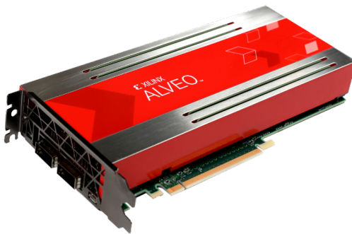
Figure 2.16: A Xilinx ALVEO computing accelerator card with two SFP slots (left side of card) for Gigabit Ethernet and a PCIe x16 connector (bottom of card) to be plugged into a computer. The card is equipped with an FPGA (covered by the red housing) and internal cooling. a
