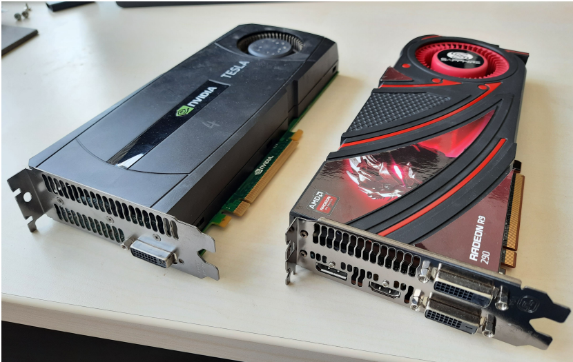
Figure 2.11: An Nvidia Tesla K40c computing GPU (left) and an AMD Radeon R9 290 consumer-grade GPU (right)
