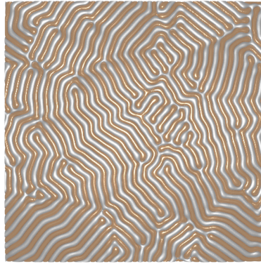
(b) Starting from an eutectic seed with anisotropic \alpha -Al and isotropic \theta results in a lamellar structure.
