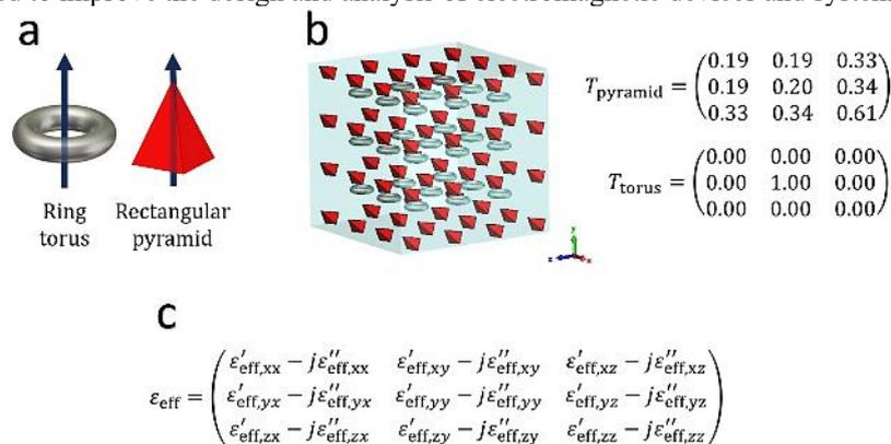
**Fig. 1.** (a) Examples of inclusions with non-spherical or non-ellipsoidal shapes and their basis orientation direction, (b) material with anisotropic-oriented inclusions according to their second-order orientation tensor  $T$ , (c) permittivity tensor, which describes the anisotropic behaviour of a material in response to an electric field.
