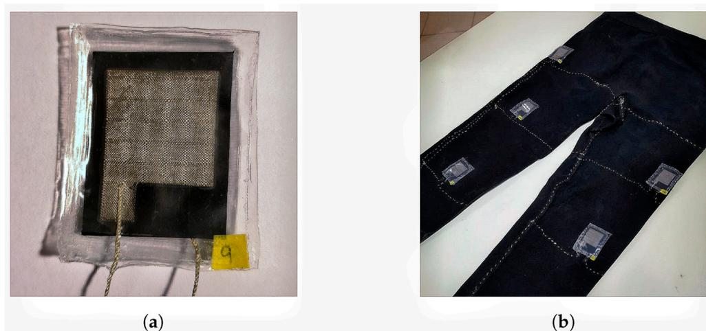
**Figure 5.** (a) Sample of the textile pressure sensors self-manufactured by [43].; (b) textile pressure sensors attached to expandable fabric pants [43] (Reprinted with permission from [43], 2023 MDP).
