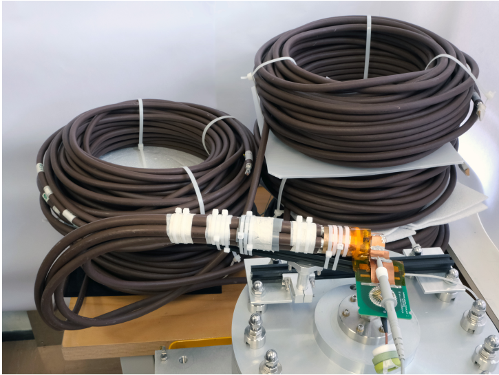
Figure 4.1: Five 50\ \Omega coaxial cables used as a replacement load for a short-circuit terminated kicker system with a characteristic impedance of 10\ \Omega . The cables are connected in parallel on the input side, individually short-circuit terminated, and have a matched one-way signal propagation time of 208 ns.
