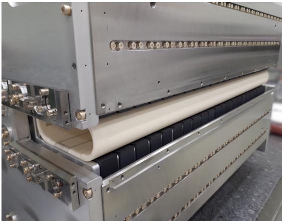
Figure 1.3: Photo of a transmission line type kicker magnet [10].
