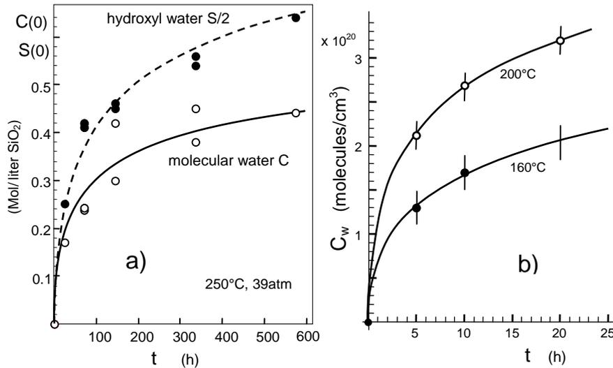
**Fig. 1** a) Molecular water (C) and hydroxyl water content (S/2) at the surface of silica for 250°C at an equilibrium vapour pressure of 39atm from [1], b) Solubility of water at silica surfaces under saturation pressure by Helmich and Rauch [3], water molecules per cm<sup>3</sup> vs. soaking time  $t$ .
