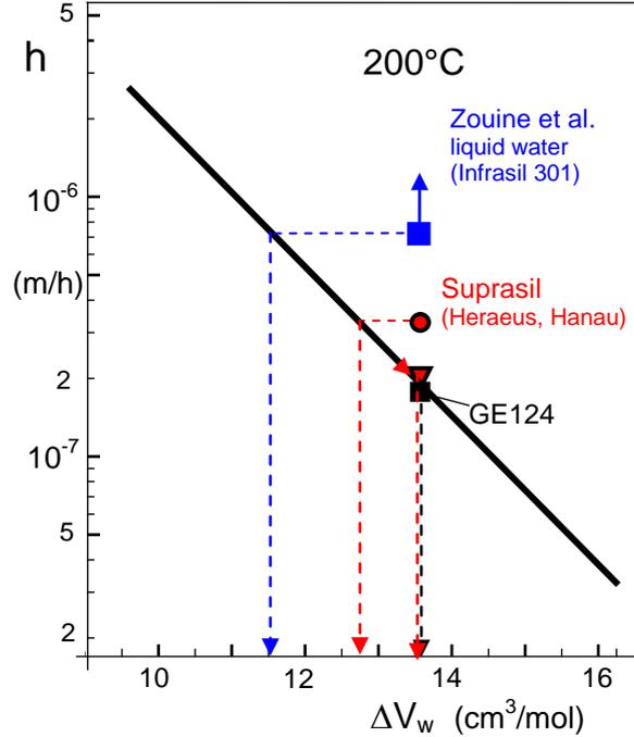
**Fig. 6** Mass transfer coefficient computed by eqs.(15) and (16), compared with measured data from Fig. 2b on Infrasil 301 and Suprasil.
