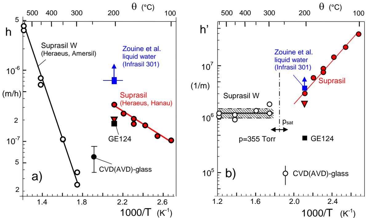
**Fig. 2** a) Mass-transfer parameter  $h$  as a function of temperature; b) mass transfer coefficient in the form of  $h'=h/D$ .
