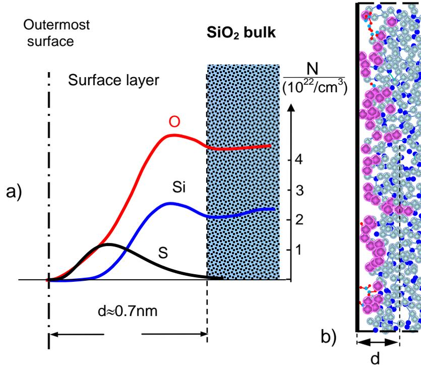
**Fig. 3** a) At a free silica surface water reacts nearly instantaneously with under-coordinated silica species in a thin surface layer of about 0.7 nm thickness; per 2-coord O (and 3-coord Si) 1 H<sub>2</sub>O molecule reacts to SiOH (curves according to Mahadevan and Garofalini [12]), b) surface layer on silica (pink: H, grey: O, blue: Si).
