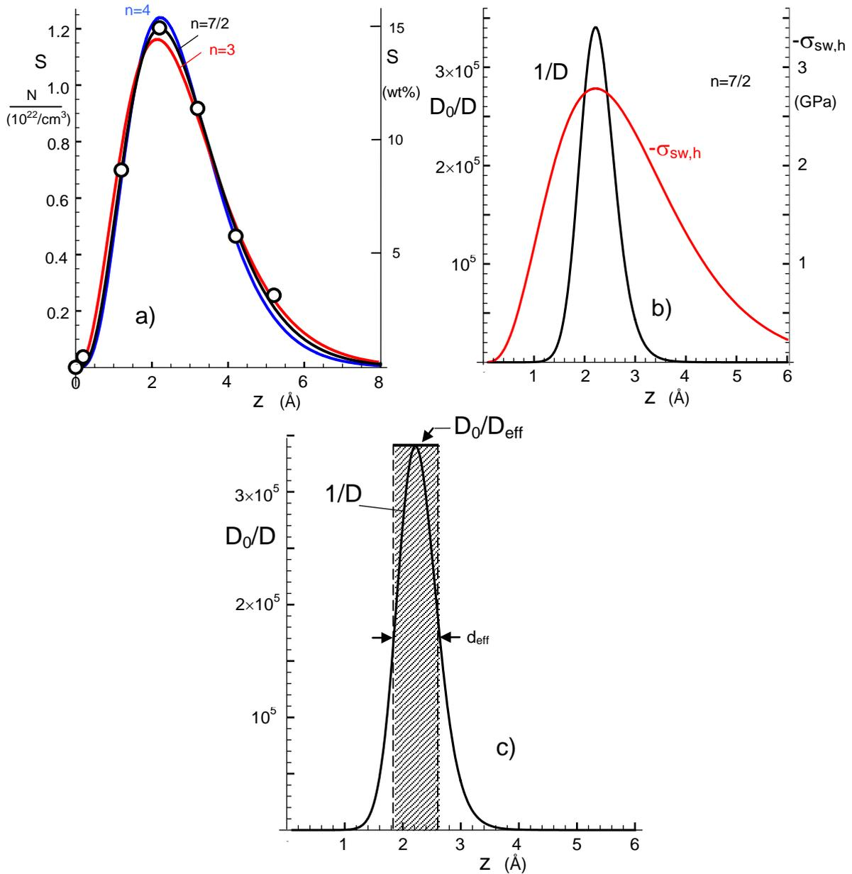
**Fig. 5** a) Data for the application of a least-squares fitting procedure (circles) and two results (curves), b) diffusivity and swelling stresses for  $n=7/2$  at 200°C, c) replacing the distribution of the diffusivity by a constant effective diffusivity  $D_{eff}$  over the effective width  $d_{eff}$ .
