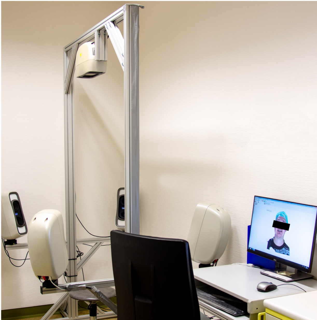
Figure 1. Vectra-M5 360 (Canfield Scientific Inc., Fairfield, NJ, USA) System is a three-dimensional stereophotogrammetry camera system that consists of five cameras.
