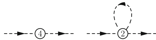
Fig. 133 Self-energy diagrams at \mathcal{O}(q^4) . Vertices derived from \mathcal{L}_{2n} are denoted by 2n in the interaction blobs
