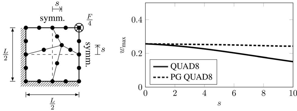
**FIGURE 3** Resulting maximum vertical displacement  $w_{\max}$  for the clamped square plate example, when employing eight-node Bubnov–Galerkin (QUAD8) or eight-node Petrov–Galerkin (PG QUAD8) elements.
