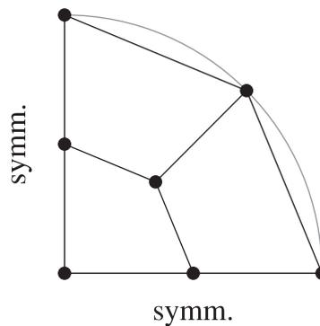
**FIGURE 6** The mesh used in the circular plate example.
