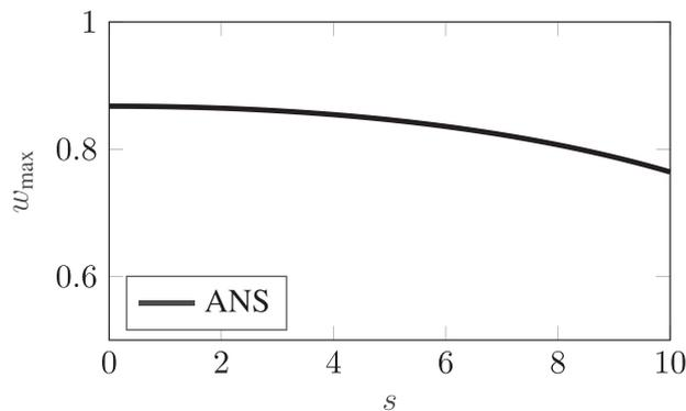
**FIGURE 2** Resulting maximum vertical displacement  $w_{\max}$  for the clamped square plate example, when employing four-node ANS (ANS) elements.
