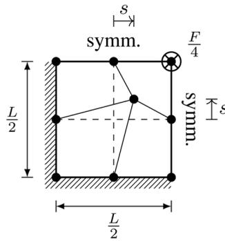
**FIGURE 1** The mesh of the clamped square plate example depending on a mesh distortion parameter  $s$ .
