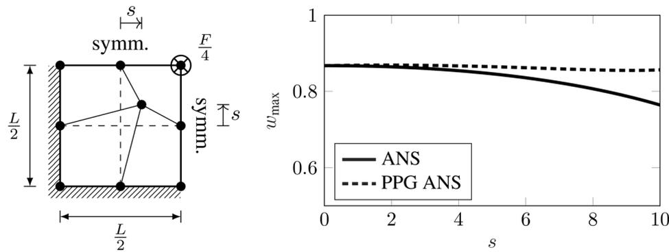
**FIGURE 5** Resulting maximum vertical displacement  $w_{\max}$  for the clamped square plate example, when employing four-node Bubnov–Galerkin ANS (or four-node partial Petrov–Galerkin ANS (PPG ANS) elements.
