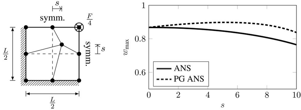
**FIGURE 4** Resulting maximum vertical displacement  $w_{\max}$  for the clamped square plate example, when employing four-node Bubnov–Galerkin ANS (ANS) or four-node Petrov–Galerkin ANS (PG ANS) elements.
