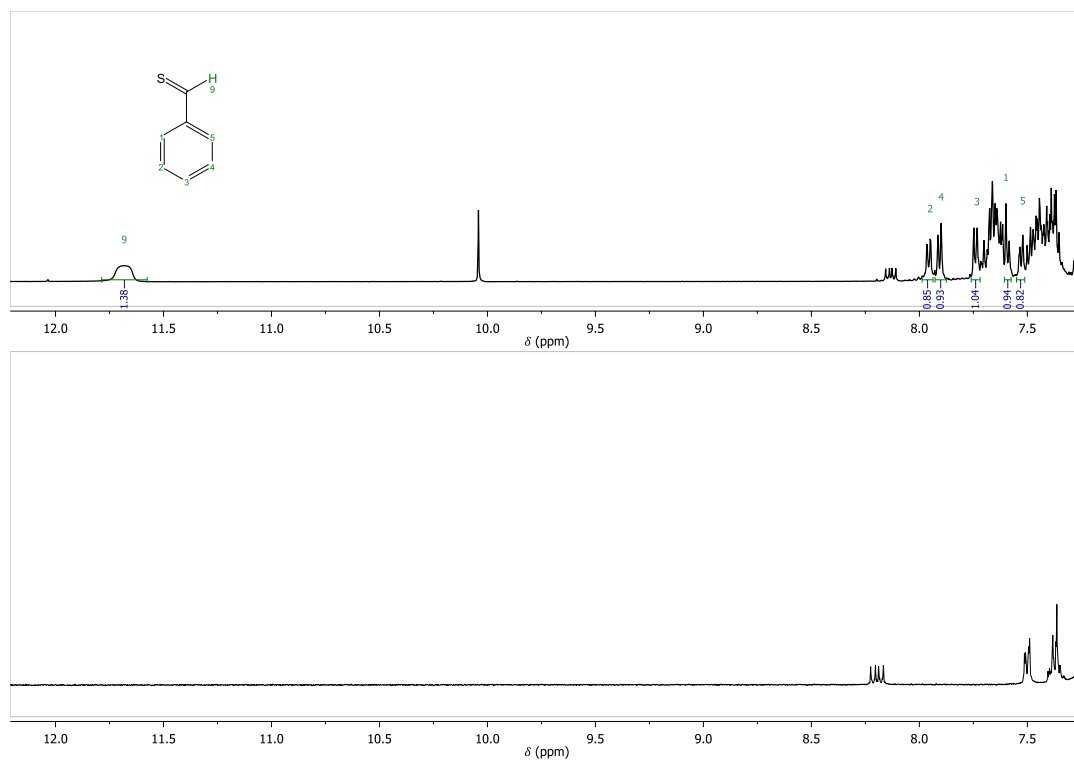
Figure 5.15.: 1 H NMR spectra of 2d compared at room temperature (bottom spectra) and 100 °C (upper spectra).
