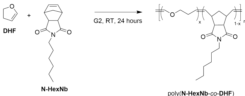
Figure 2.7.: Reaction scheme of the copolymerisation of DHF with a norbornene derivative.
