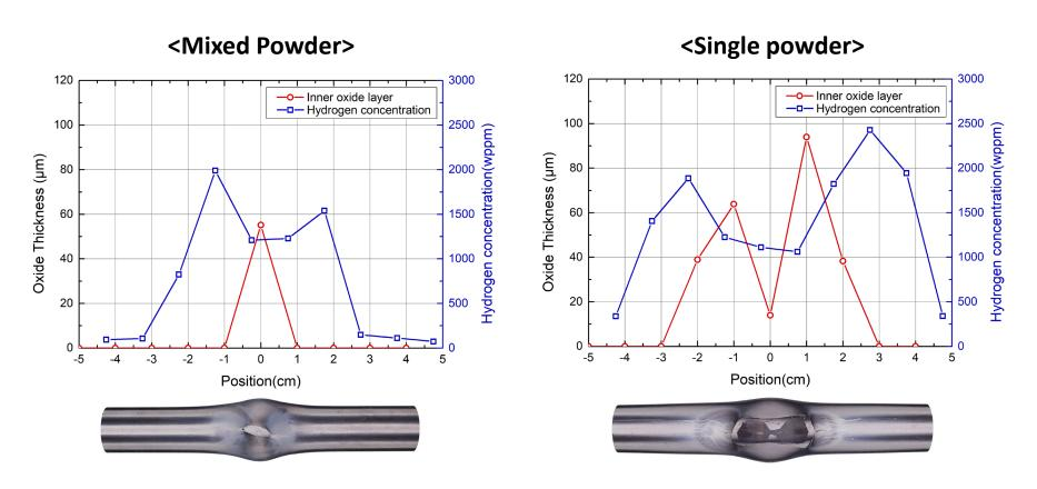
The larger the hole, the larger the inner oxidation and secondary hydride formation
