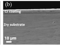
Fig. (a) Cladding tube and (b) cross-sectional of Cr-coated Zry cladding manufactured by MNF. (As-received)
