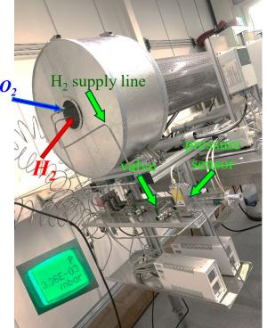
$V_{H2} = V_{hot clad} + V_{cold supply} = 133 \text{ cm}^3 + 20 \text{ cm}^3$
