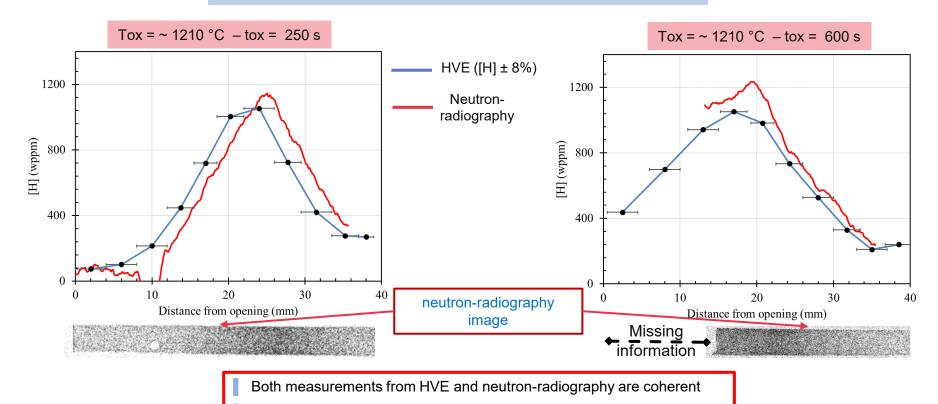
The hydrogen maximal content can be slightly be underestimate by HVE
