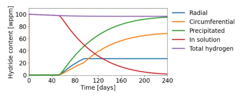
Pre-test calculations with the TESPA-ROD code: Prediction of the hydrogen behaviour at the hottest position of the central rod #01 during the test
