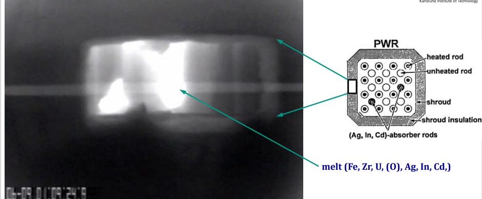
melt <u>viscosity</u> depends on temperature T and volume fraction of <u>ceramic precipitates</u> f
