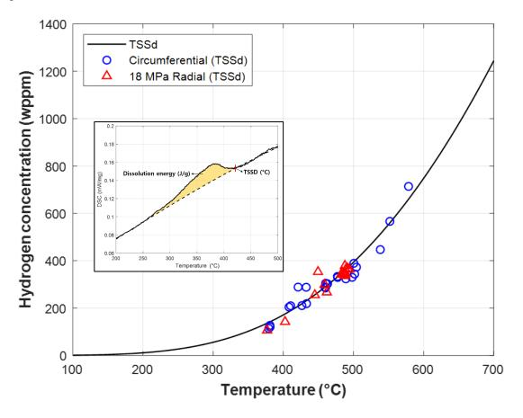
Measured TSSd fits very well with the theoretical value<sup>[6]</sup>, and there was no difference in TSSD between the radial hydride and the circumferential hydride.
