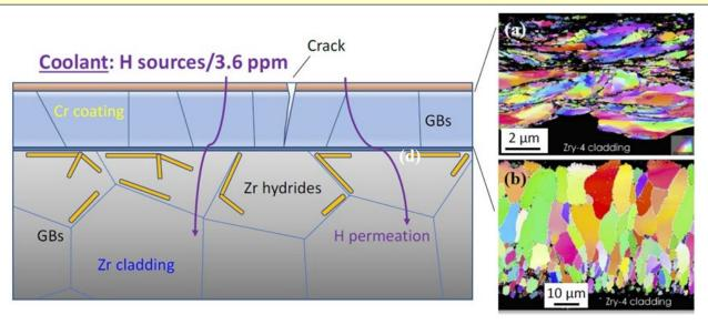
The multimodal comparative post irradiation examination (PIE), supported by a DOE GAIN Voucher, will aim at gaining unique insights into the hydrothermal corrosion effects and hydrogen transport mechanisms governing the formation of embrittling Zr hydrides in various Cr-coated ATF claddings concepts provided by Westinghouse Electric Company LLC (WH).
