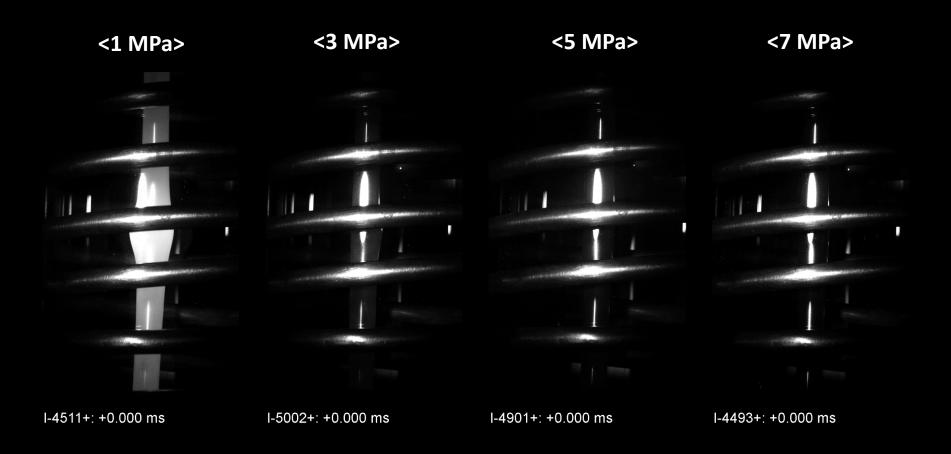
The higher the rod pressure, the more particles were dispersed
