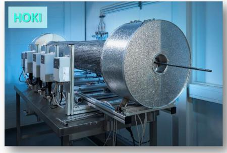
Apparatus for in-situ neutron radiography experiments under defined mechanical load and temperature
