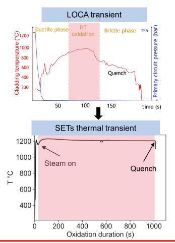
Tests in oxidizing environment (50% Ar + 50% H<sub>2</sub>O) at ~1200 °C
