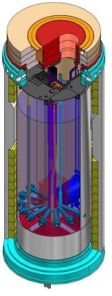
**Objective**: Provide comparative data on the irradiation induced creep of current Zr alloys and Cr coated samples under steady state conditions
