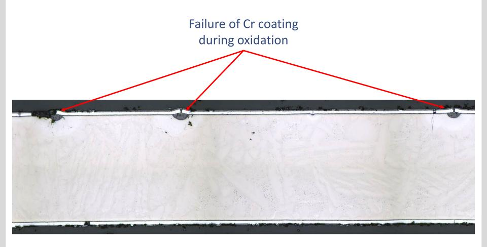
Indication for too thick Cr coating resulting in thermo-mechanical mismatch?
