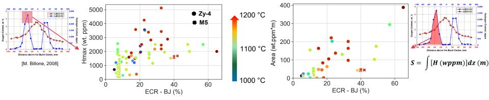
Data obtained from LOCA tests in literature regarding secondary hydriding on unirradiated cladding ( JAEA, EDF, CEA, KIT, IRSN)
