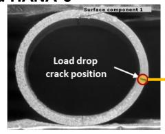
Change of major load drop through-wall crack position>
