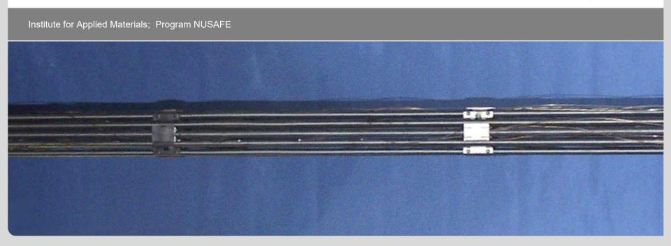
Melt relocation: rivulets and droplets in CORA-PWR tests
