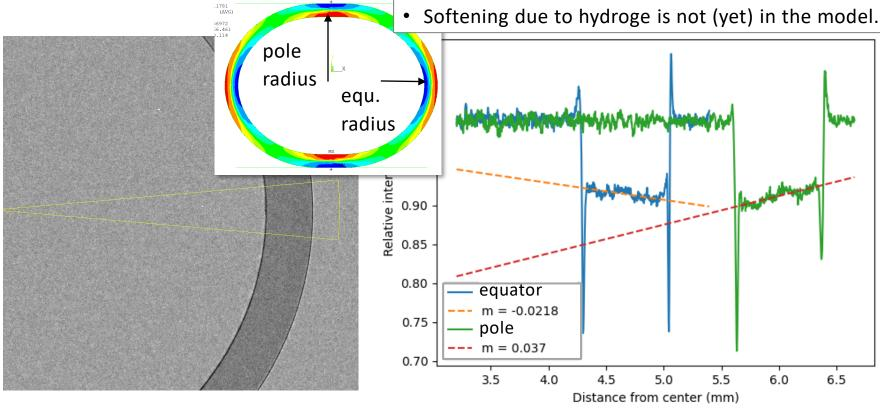
neutron image of 200 wppm hydrogen sample with region of interest (equator), angular integration
