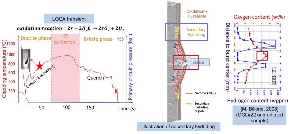
$Ballooning \rightarrow Burst \rightarrow Steam \ ingress \ in \ the \ inner \ side \ of \ the \ cladding \rightarrow oxidation \rightarrow secondary \ hydriding$
