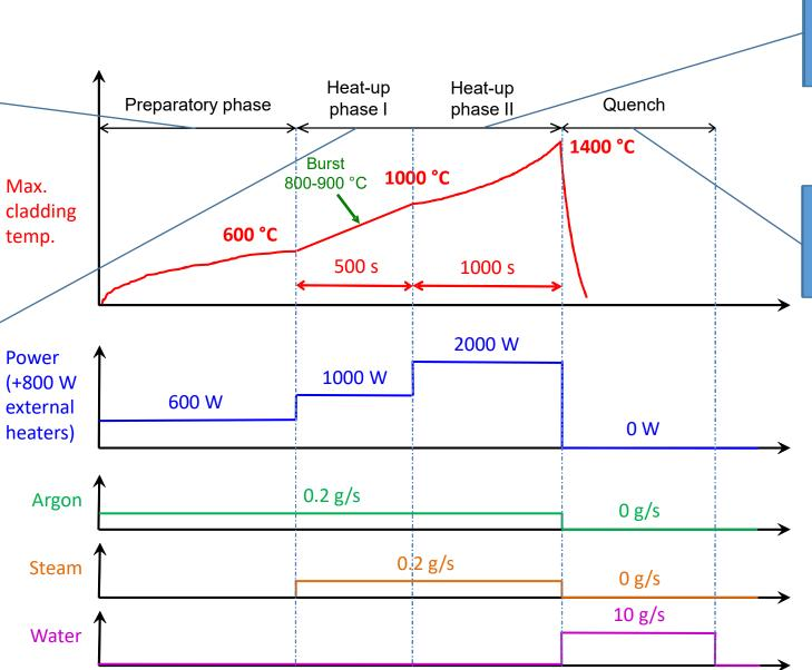
further heat-up with increased power, target temperature of 1400 °C
