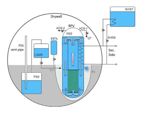
iPWR characterized by the use of several passive systems, a dry containment and an electric power of about 300 MWe,
