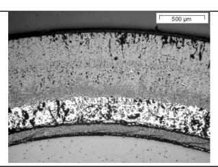
PWR QUENCH-06 (Zry-4), rod #12, 950 mm: melt captured between clad oxide and pellet
