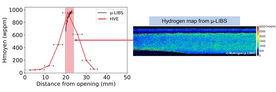
μ-LIBS analysis and HVE measurements are consistent
