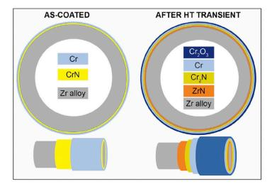
**Fig. 19.** The design of the multicomponent cladding that avoids Zr–Cr eutectic reaction and material inter-diffusion during high-temperature transients. Nitrogen is released from CrN to form ZrN above 975°C.
