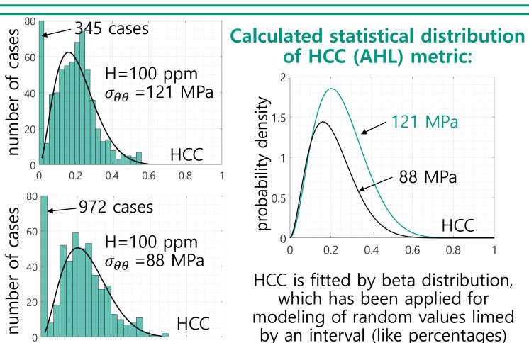
Hydrogen Continuity Coefficient (HCC) or Accumulated Hydride Length (AHL):
