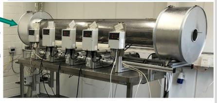
HOKI oven with axial temperature profile:  $T \approx 450$  °C along the length of  $\approx 1250$  mm
