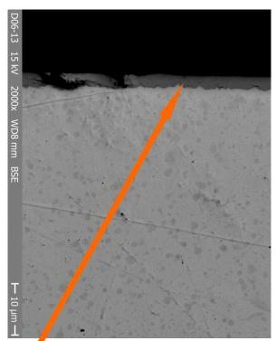
outer ZrO<sub>2</sub> 2.4 μm (formed during 4.5 days at 450 °C) corresponds 0.3% O in whole sample, what was confirmed also by hot extraction
