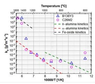
Fitting functions for weight gain provided by J. Stuckert
