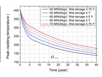
Dry storage simulation thermal analysis result
