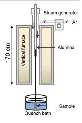
Tests in oxidizing environment (50% Ar + 50% H<sub>2</sub>O) at ~1200 °C
