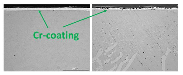
Zr1Nb+Cr (before oxidation, 1200°C / 15 min)
