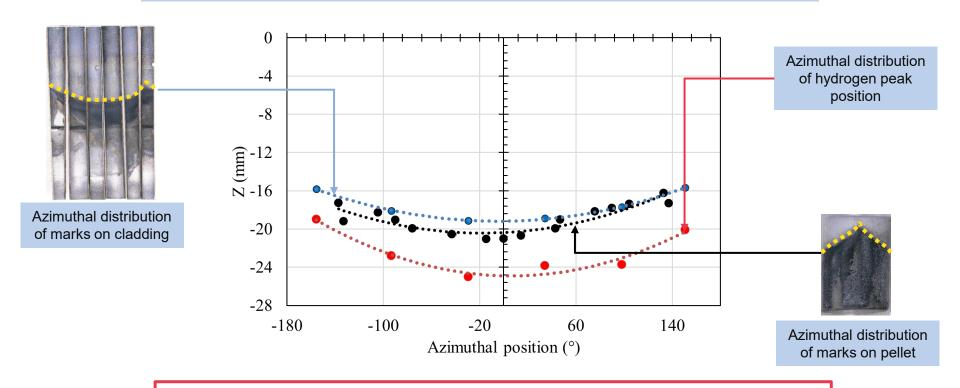
The marks on both the inner cladding surface and pellet surface are coherent
