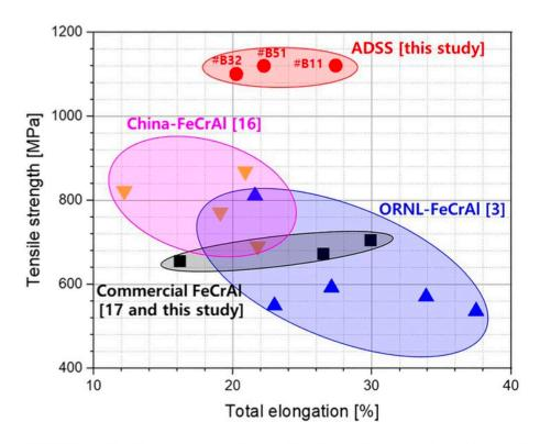
**FIGURE 8** Tensile strength as function of total elongation of alumina-forming duplex stainless steel (ADSS) alloys, wrought FeCrAl model alloys, and commercial FeCrAl alloys [Colour figure can be viewed at wileyonlinelibrary.com]
