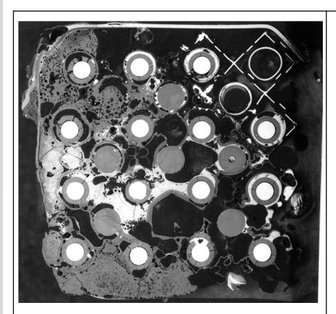
PWR CORA-15 ( $T_{pct} \approx 2370 \text{ K}$ ), elevation 480 mm: melt collection at spacer grid
