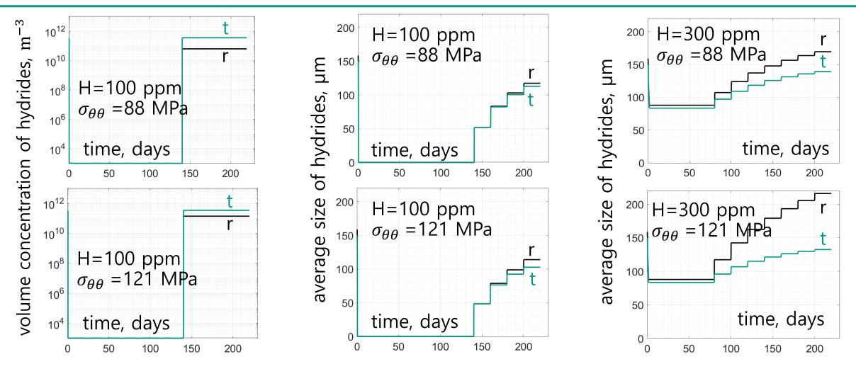
The morphology of the hydrides is a function of their initial state in the 300 ppm samples, <u>but not</u> in the 100 ppm samples.
