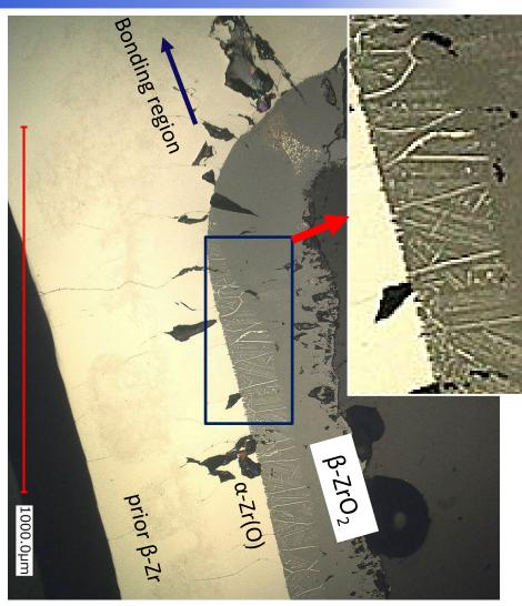
Suggests that a large temperature gradient of more than 180 °C occurred in the 15 mm length between the neck region and burst level.
