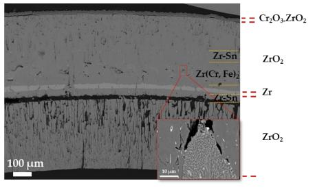
Double-sided steam oxidation test at 1400 °C for 360s.
