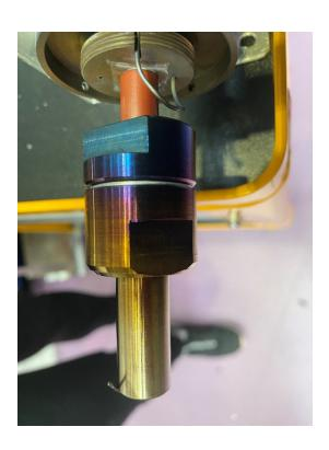
new leak-tight sample holder with aluminium sealing ring
