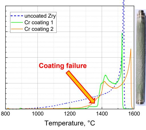
Faster oxidation of coated samples after coating failure compared to Zry in <u>single-rod</u> experiments with high heat losses!
