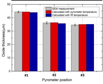
Oxide thickness calculated with temperature profile of pyrometer and IR camera were consistent with SEM measurement
