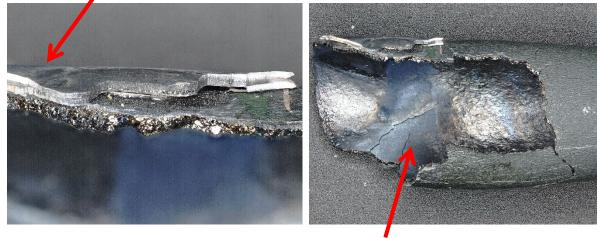
oxidation of inner cladding surface
