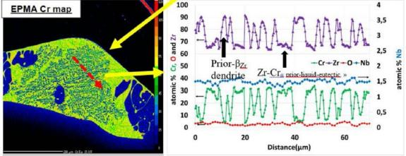
One-sided steam oxidation test at 1400-1405 °C for 100s with water quenching to RT.
