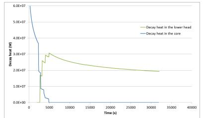
Decay heat in the reactor core and the corium in the lower head.
