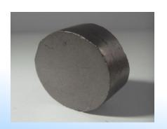
UN pellet produced by spark plasma sintering.
