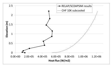
Maximum heat flux at the external surface of the RPV wall calculated by RELAP/SCDAPSIM.
