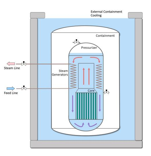
iPWR characterized by a submerged containment and electric power of about 60 Mwe
