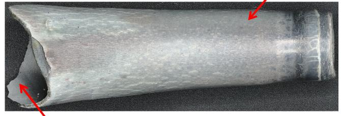
oxidation of inner cladding surface
