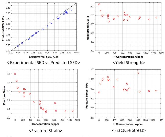
• SED and fracture strain decreases with the H concentration while yield strength and fracture stress do not have a strong correlation with the H concentration.
