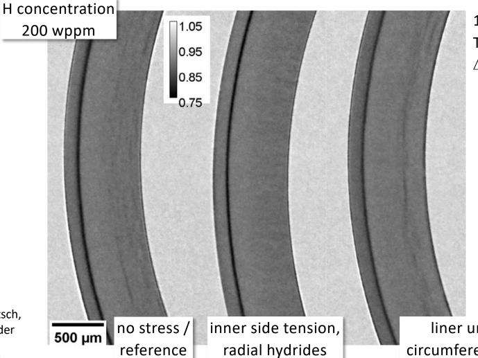
1 cycle  $T_{max} = 400$ °C  $\Delta T_{cooling} = 30$ °C/h
