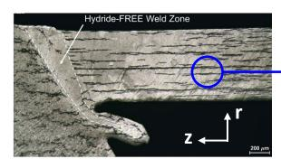
Axially parallel grain boundaries and intergranular hydride interface
