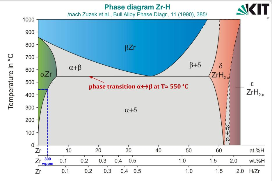
hydriding of claddings should be performed at T<550  $^{\circ}\text{C}$  to avoid the phase transition
