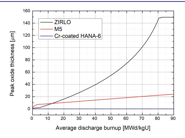
Accident tolerance comes from steady state corrosion resistance: Steady-state
