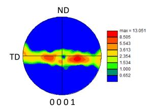
Theoretically, it was considered that circumferential hydride precipitates at basal plane and radial hydride precipitates at the prismatic plane.<sup>[5]</sup>
