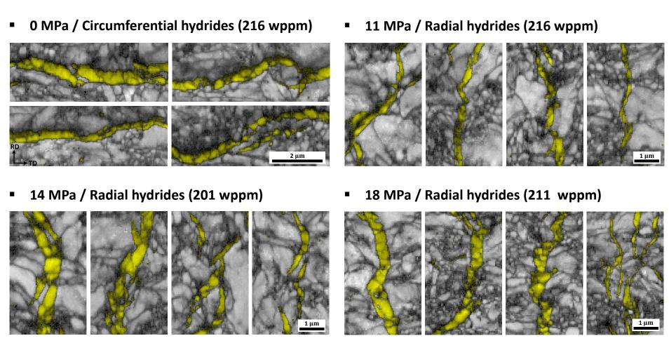
To exclude the effect of the undissolved circumferential hydride on the precipitation of the radial hydride, specimens with low H concentration (~200 wppm) were prepared.
