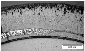
PWR QUENCH-15 (ZIRLO), rod #17, 1000 mm: melt captured between clad oxide and pellet
