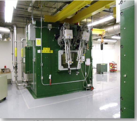
12-inch steel shielding 7'W x 5'D x 12'H inside dimensions
