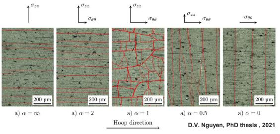
Cracks initiation independent of biaxiality state (however, it affects cracks' orientation and distribution)
