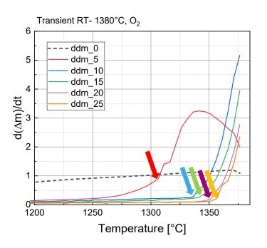
Transition time from protective to non-protective coating increases with Cr thickness for all three test series
