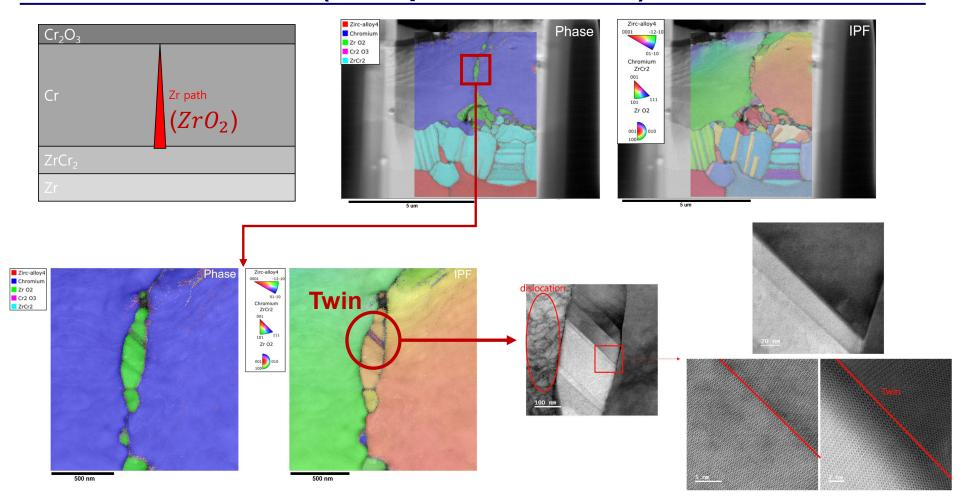
• Sign of strong tensile stresses near  $ZrO_2$ : The elastic stress fields near the  $ZrO_2$  may lower the local chemical potential, thereby accelerating the oxygen diffusion along the grain boundaries via steeper diffusion potential gradient. This may hold a clue to understanding the eccentrically fast oxygen diffusion across the Cr thickness upon the loss of its protection.
