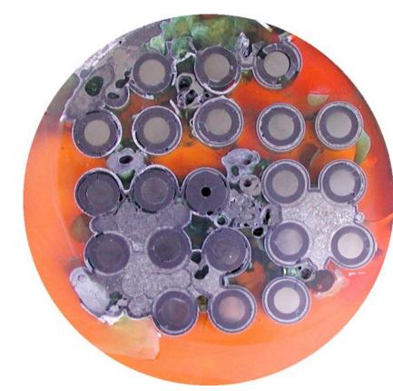
PWR QUENCH-11 ( $T_{pct} \approx 2100 \text{ K}$ ), elevation 837 mm: formation of large molten pools below the bundle hot region
