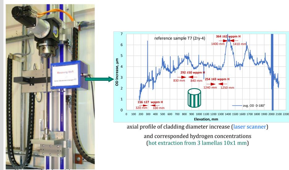
profilometry of clads with laser scanner (thermal expansion ±0.3 μm for ±5 °C)
