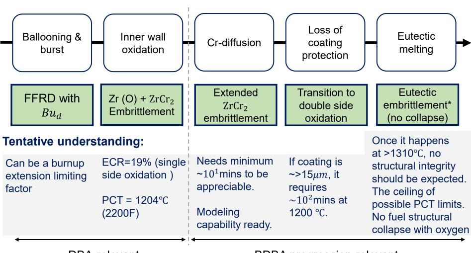
DBA-relevant (i.e., ECCS Criteria 10 CFR 50.46) BDBA progression-relevant (DEC condition)
