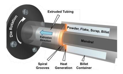
Extrusion process with a rotating die
