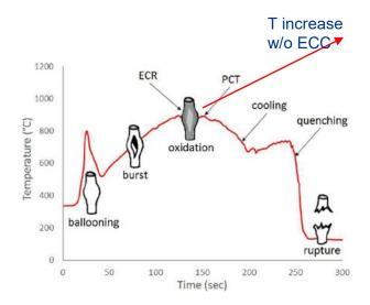
Need to decrease the rate and the total amount of heat generated and the build-up of hydrogen generated from cladding oxidation in hight temperature steam
