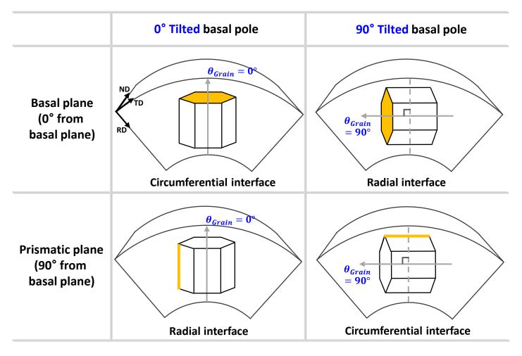
While exhibiting the same interface plane, each interface is available to result in the different orientation (radial / circumferential) of the hydride according to the tilted angle of Zirconium.
