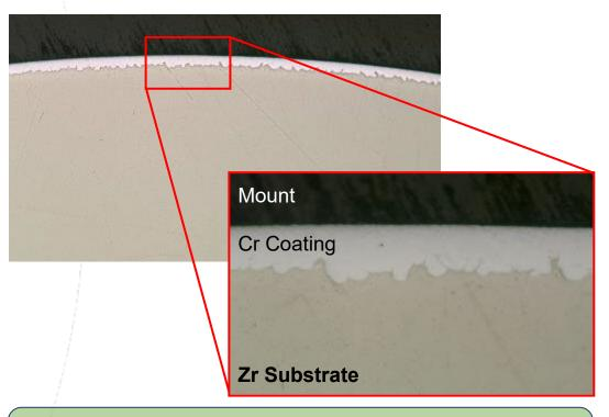
Excellent cold sprayed Cr coating integrity with complete protection of substrate
