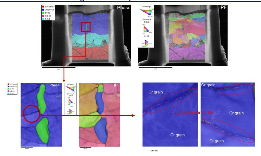
• Sign of oxygen ingression through Cr grain boundary and early formation of  $ZrO_2$ :  $ZrO_2$  formation may occur before Zr reaches the top surface  $(Cr_2O_3)$ . Zr may pick up oxygen from the  $Cr_2O_3$  present in the grain boundaries and becomes  $ZrO_2$  along its way to the top.
