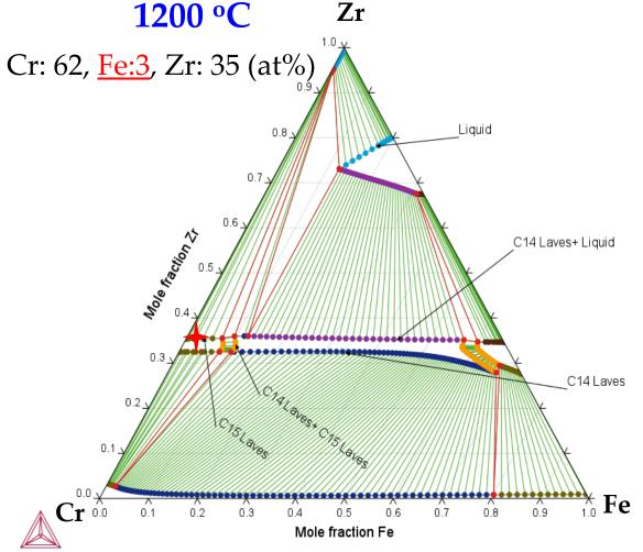
1200 °C: C15 Laves phase of Zr(Cr, Fe)<sub>2</sub> 1300 °C: C14 Laves phase of Zr(Cr, Fe)<sub>2</sub>.. Fe enrichment
