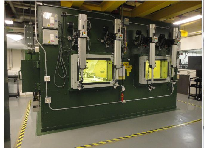
12-inch steel shielding 10'W x 5'D x 12'H inside dimensions
