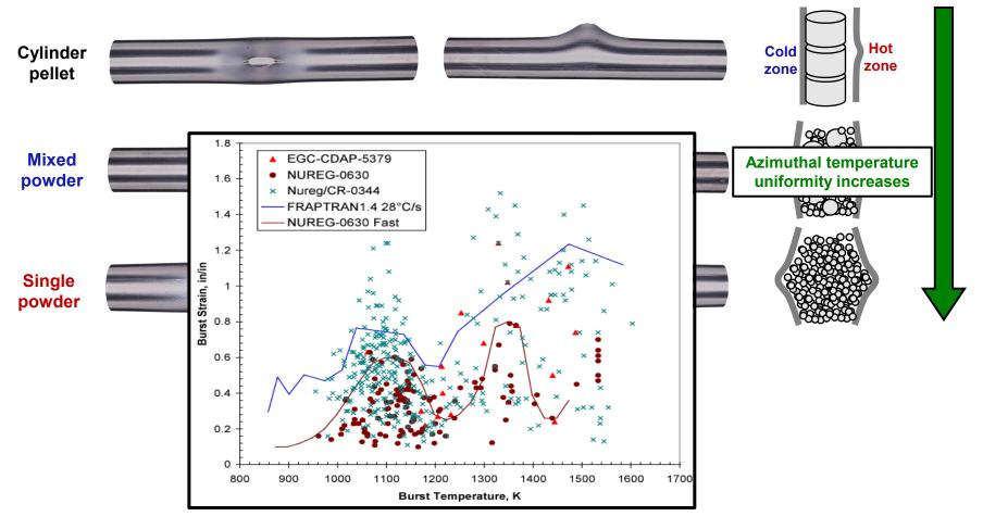
The size and distribution of fragmented fuel have a significant effect on burst behavior
