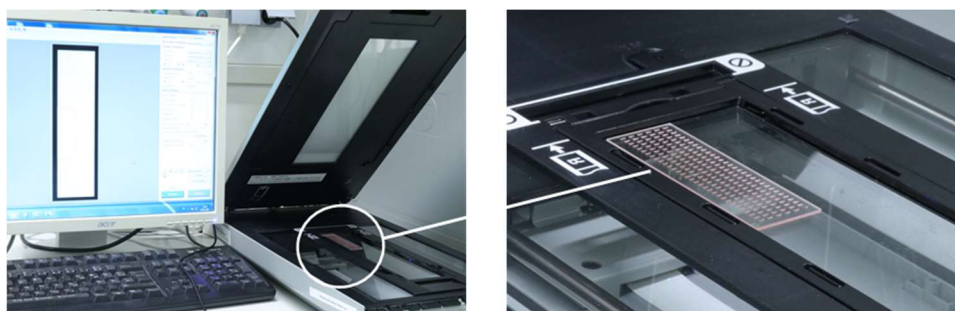
Figure 16: Document scanner as imaging option for Droplet Microarrays. Adapted from WIEDMANN et al. [2]
