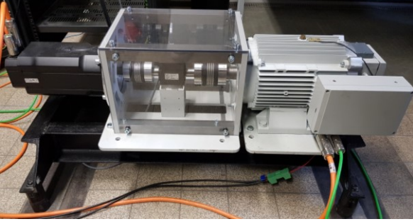
Fig. 9. Testbench with LTI - LSH-127-4-30-560/T4,1R (left) as load machine and the EESM DUT on the right.
