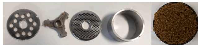
Fig. 2. Inner setup of meat grinder and size reduced Reed Canary Grass (RCG) (Biomass H).
