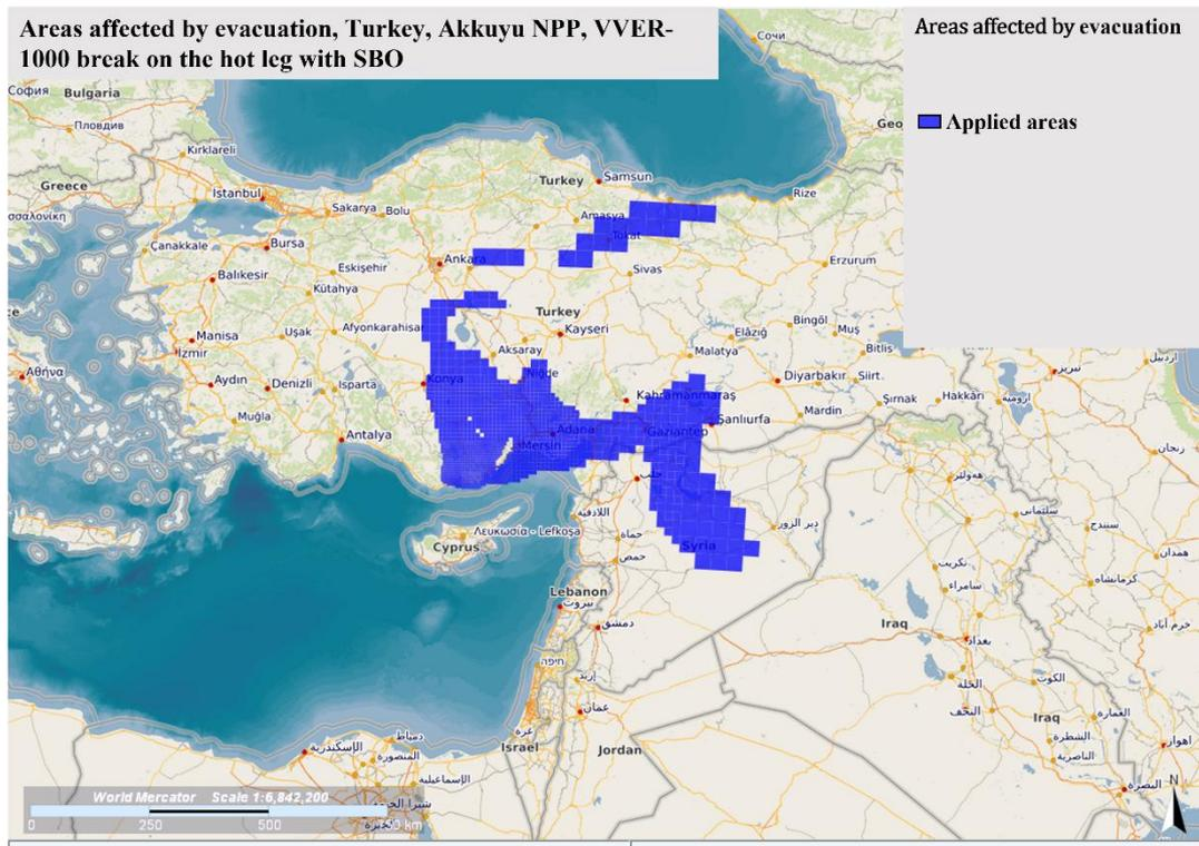
Figure C.2- 16: Simulated evacuated regions as early emergency applications at the end of 10th day of radiological dispersion for the hot leg accident case
