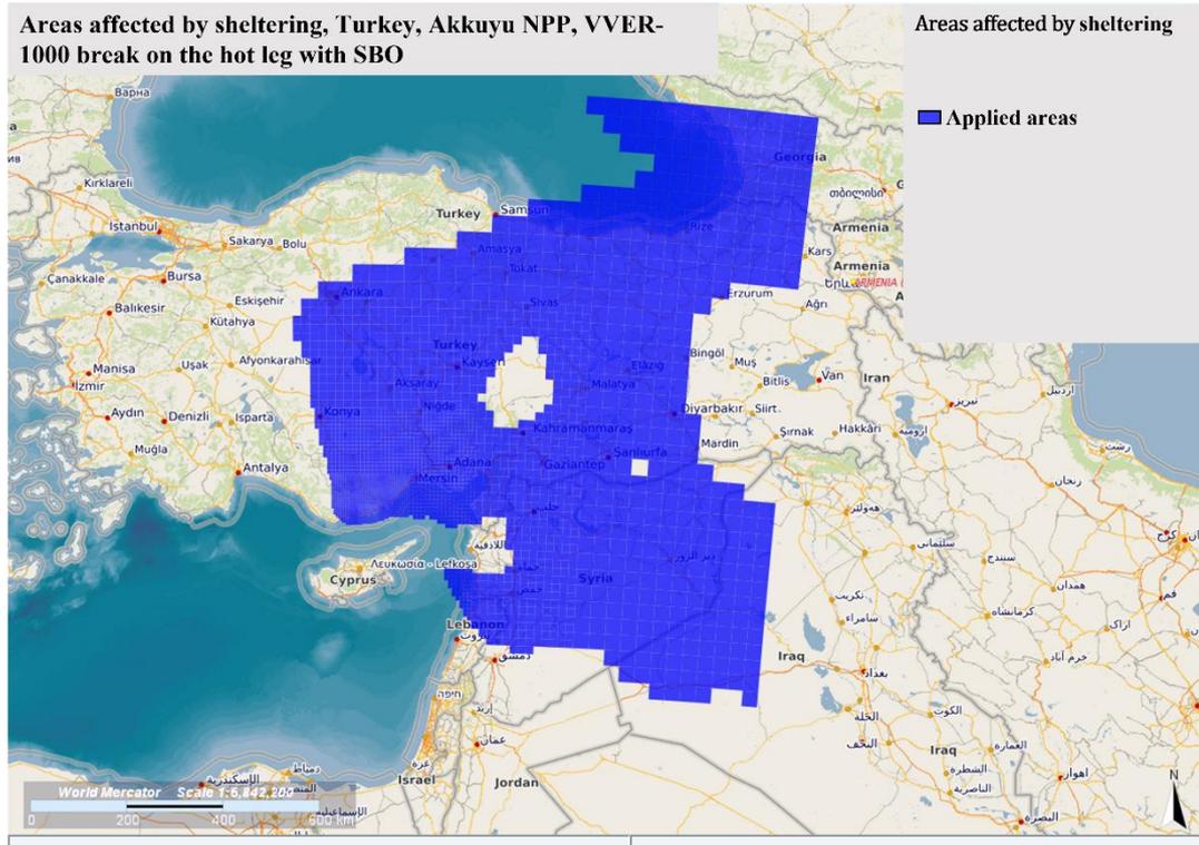
Figure C.2- 15: Simulated sheltered regions as early emergency applications at the end of 10th day of radiological dispersion for the hot leg accident case
